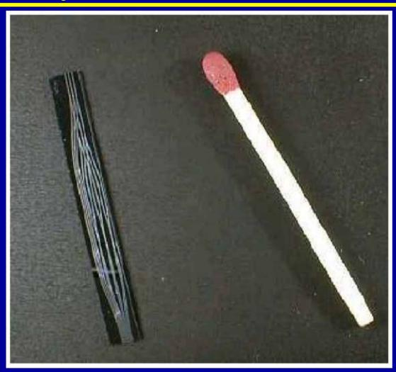
Produced by LETI with silica-on-silicon etching technique
