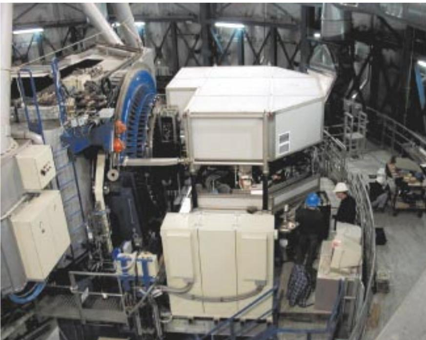
*Figure 1: This aerial view of the Nasmyth platform of Kueyen at the end of the integration shows UVES with the top of its enclosure partially lifted to have access to the table where the various components are mounted. The bar connecting the enclosure to the telescope fork is for safety in case of earthquake.*
