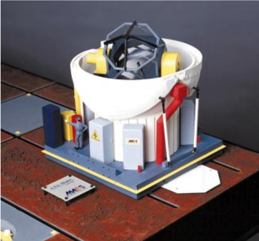
Figure 3: A model of an Auxiliary Telescope during Observations. The 1.8-m telescope (with an Alt-Az mount like the Unit Telescopes) is rigidly anchored to the ground by means of a special interface. The light is directed via the Coudé Optical Train to the bottom of the Telescope. From the Coudé Relay Optics it is sent on to the underground Delay Line Tunnel
