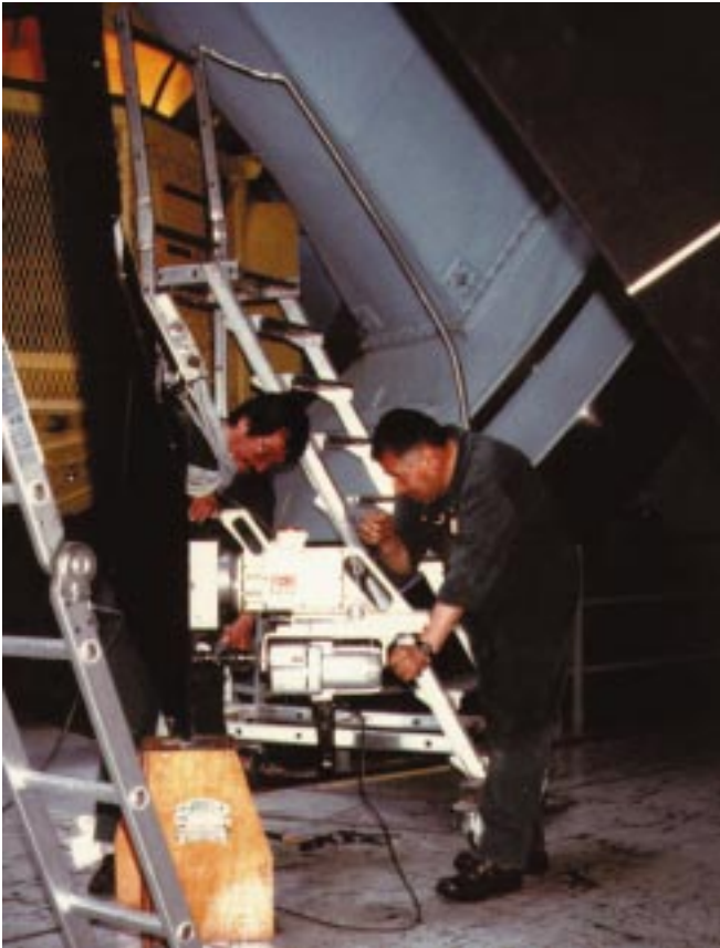
Figure 1: Hard and heavy mechanical work at the observing floor: H. Quichón and P. Alvarez are remachining the spider of the infrared f/35 secondary at the observing floor of the 3.6-m dome.
