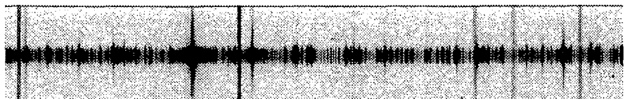
Figure 1: Two-dimensional image of the Th-Ar exposure centred at 6470 Å.
