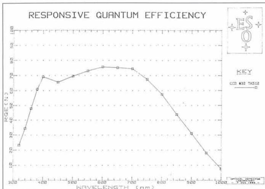
Figure 2: R.Q.E. of CCD #32
