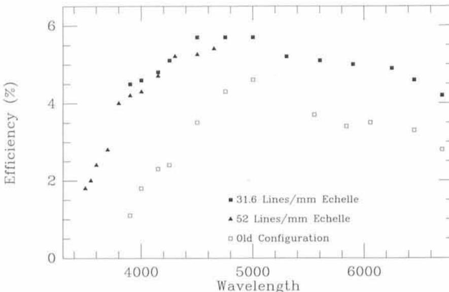
Figure 3: Overall efficiency curve for the 3.6-m telescope + CASPEC and the new Blue crossdisperser. Short Camera plus 31.6 lines/mm echelle (filled squares) and 52 lines/mm echelle (filled triangles). The results obtained with the old configuration are also shown (open squares) for comparison.
