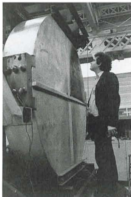
Figure 4: 1.8-m aluminium blank shortly after welding of a segment.
