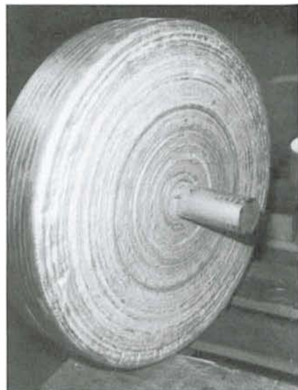
Figure 3: Build-up welded aluminium blank of 500 mm.
