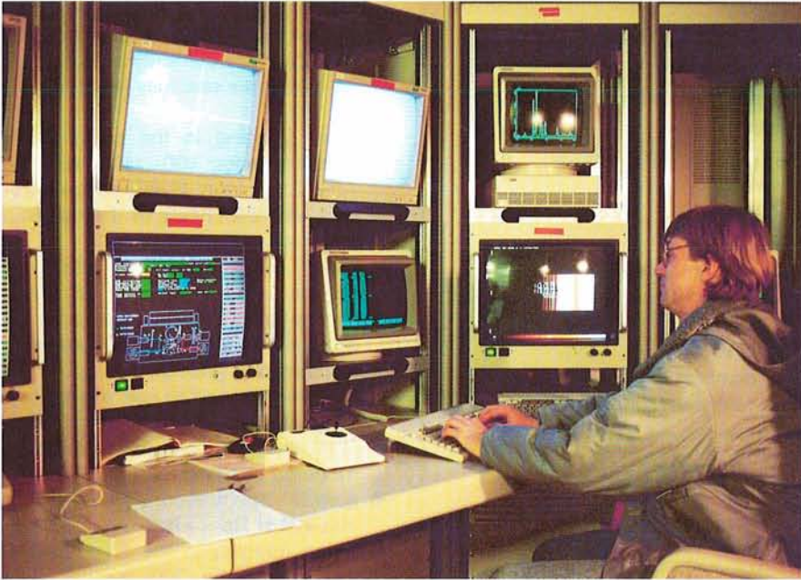
Figure 3: The "EMMI's corner" of the control room. From the left, in the lower row, a Ramtex dedicated to the user's interface displaying the layout of EMMI and the functions on line (a mouse is used to select other display options), a terminal for the exposure definition and a Ramtex displaying a long slit spectrum. In the row above two monitors for guiding and a graphic display.
