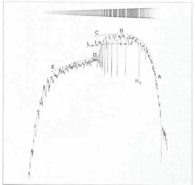
Fig. 2: The parameters  $D$  and  $\lambda_1$  of the BCD system represented on a microphotometer tracing.
