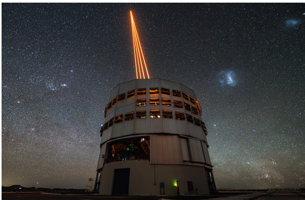
This photograph captures the Unit Telescope 4 of ESO's Very Large Telescope, located in Chile's Atacama Desert, and its four-laser system, which is used to excite sodium atoms in the atmosphere. The atoms excited by the lasers emit light that is affected by the atmosphere in the same way as the light emitted by real stars. The emitted light is collected by the telescope and can be used by the adaptive-optics system to measure the distortions introduced by the atmosphere and then to correct for them. This advanced system, combined with the excellent dark-sky conditions of the Atacama Desert, ensure the telescope can obtain extremely sharp images.
