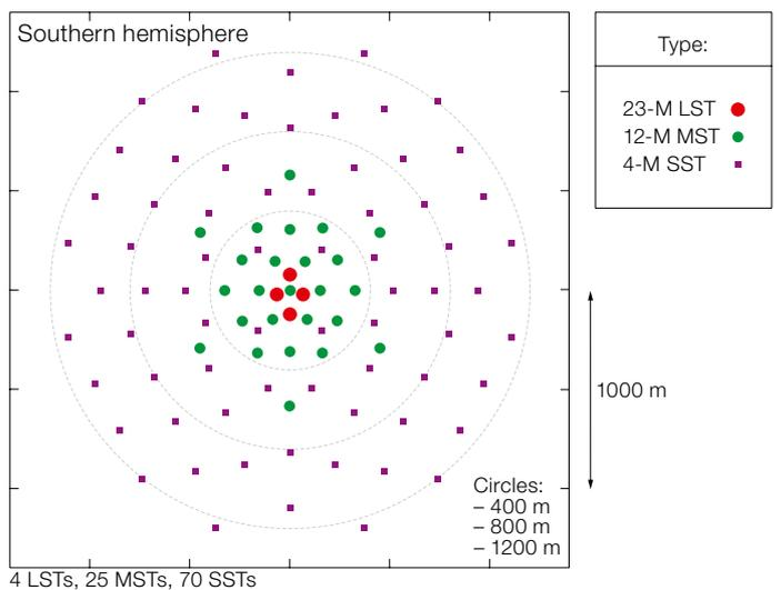
Figure 4. (Right) Layout of the southern telescope array, combining 4 LSTs, 25 MSTs and 70 SSTs.
