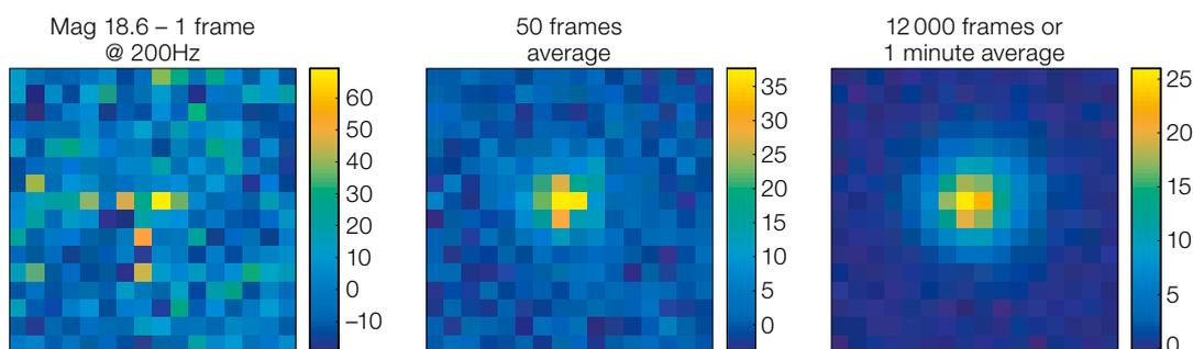
Figure 13. Individual 200 Hz frame showing the tip-tilt star signal (left), with 50 (centre) and 12 000 (right) frames averaged. The star magnitude is 18.6 and the spaxel size is 0.2 arcseconds.
