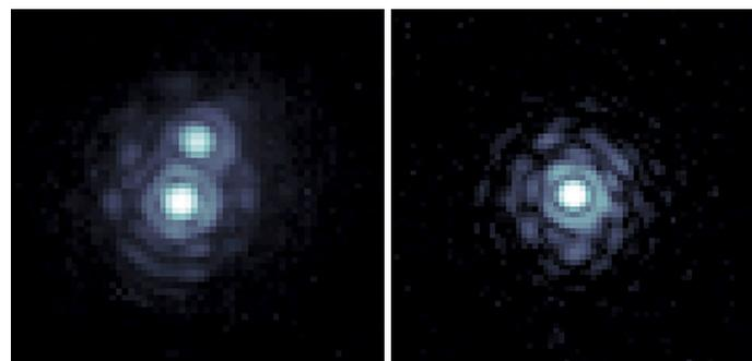
Figure 6. Left: *K*-band narrow filter image of a double star with 0.2 arcsecond separation, obtained with GRAAL MCM. Right: A bright star image exhibiting 80% Strehl ratio (also with *K*-band narrow filter). The seeing was 0.55 arcseconds at the time.
