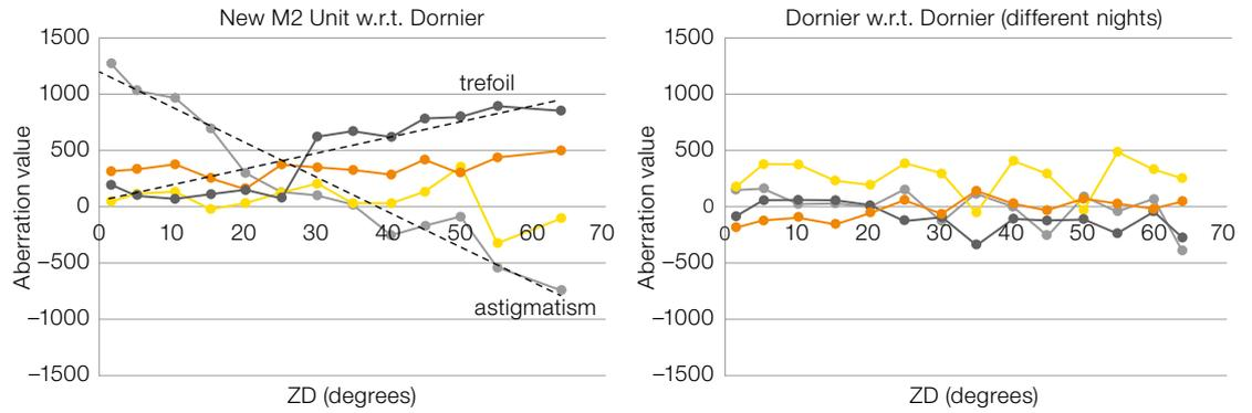
the active optics has managed this change without issue. Note that the corresponding mode amplitude applied in the DSM flattening vector has been modified to ensure that the horizontal axis crossover occurs at a typical operation airmass.
