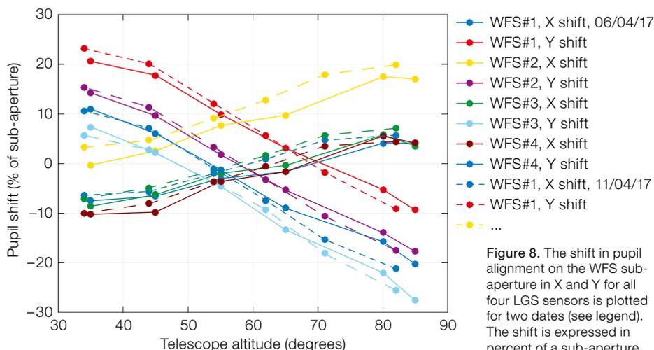
Figure 8. The shift in pupil alignment on the WFS sub-aperture in X and Y for all four LGS sensors is plotted for two dates (see legend). The shift is expressed in percent of a sub-aperture.
