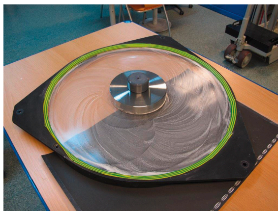
Figure 3. Photograph taken during the removal of the coating on the FORS1 LADC prisms.
