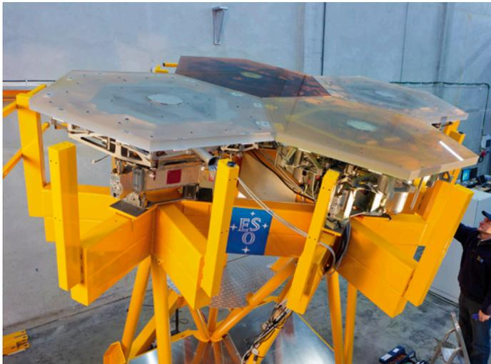
**Figure 1.** The segment test assembly in Garching. Four fully polished segments have been mounted on their supports. Edge sensors and actuators have been deployed on a number of the segments and control testing has started.
