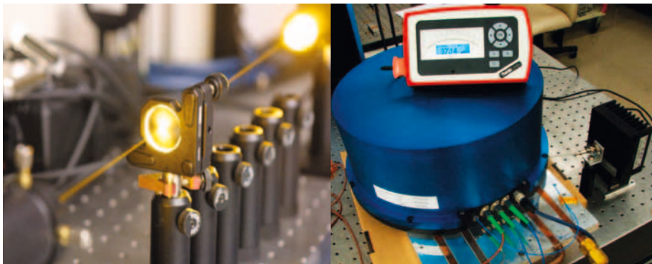
Figure 8. The optical tube assembly being developed by TNO Science & Industry. Together with the beam control and diagnostics system this assembly makes up the launch telescope system for the 4LGSF. Four similar units are mounted on the centrepiece of the UT to launch the four laser guide stars at 90 km altitude.
