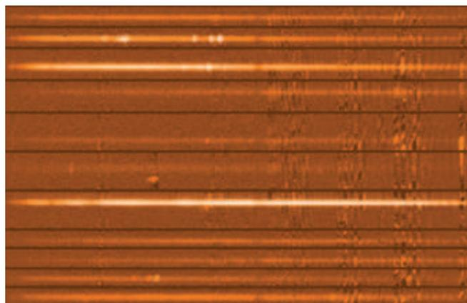
Figure 5. Same data as in Figure 4, but this time the newly proposed data reduction method has been used. The image colour cuts are identical to those in the previous figure. The significant removal of the fringing pattern, although not perfect, can be easily appreciated by comparing the two images.
