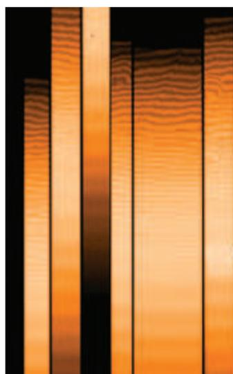
Figure 1. Fringing pattern in VIMOS MOS red data. A small portion of a flat-field exposure obtained with the LR\_red grism is shown, including spectra from six different MOS slits. The red end of the spectra is towards the top.
