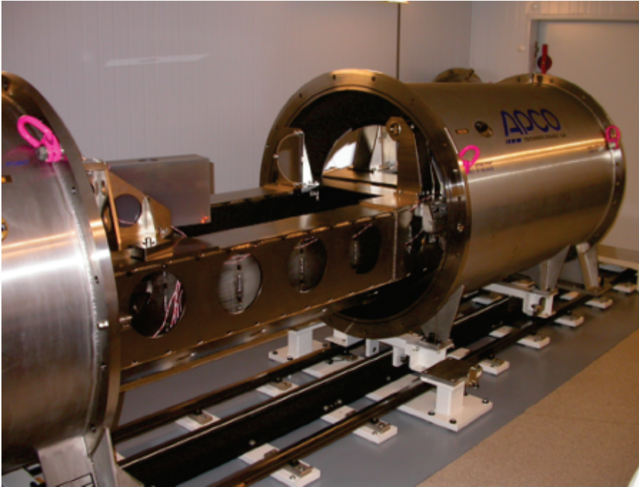
Figure 1: The HARPS spectrograph inside the air-conditioned room at La Silla just before being closed and evacuated.
