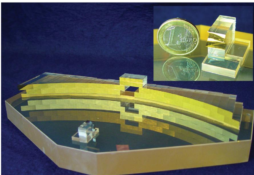
**Figure 2:** SPIFFI image slicer: The light enters through the hole in the big slicer. A stack of 32 small mirrors 'the' small' slicer – slices the image and redirects the light towards the 32 mirrors of the 'big' slicer, which rearranges the slitlets to a 31 cm long pseudo-long-slit. The small inset shows an enlargement of the small slicer.
