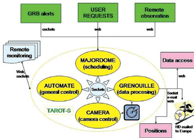
Figure 5: Software configuration of the TAROT observatory.
