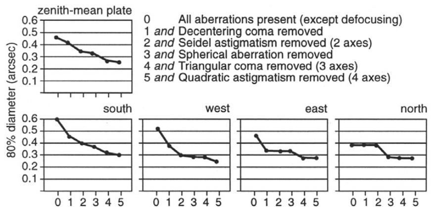
Figure 1: Results of classical Hartmann tests of the conventional ESO 3.6 m telescope in 1976, illustrating the theoretical improvement after successive removal of polynomial terms. The mean right-hand point of the functions gives the Intrinsic Quality (IQ) of the telescope. (W99)
