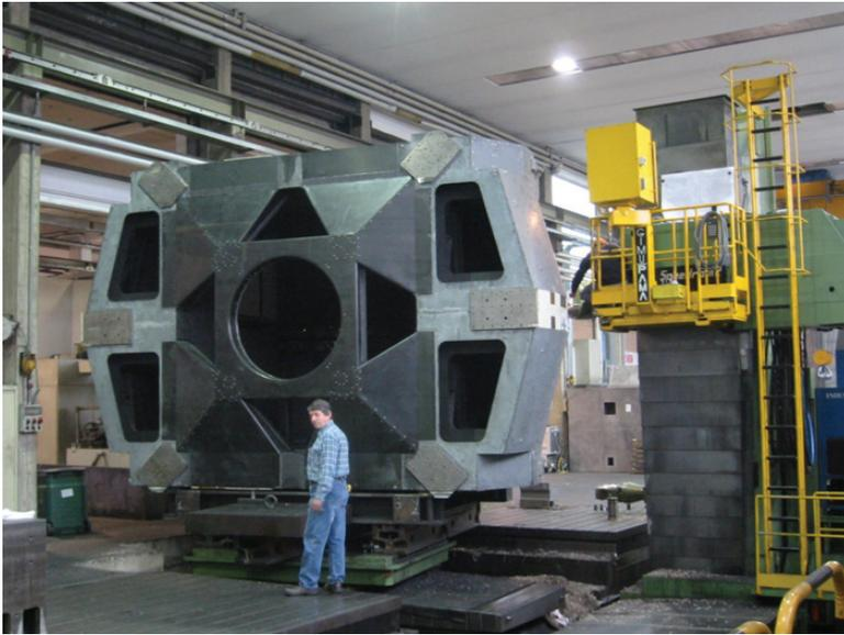
The machining of the CFRP cabin interfaces at the Galbiati factory. The machining head is working on the elevation motor attachment point.
