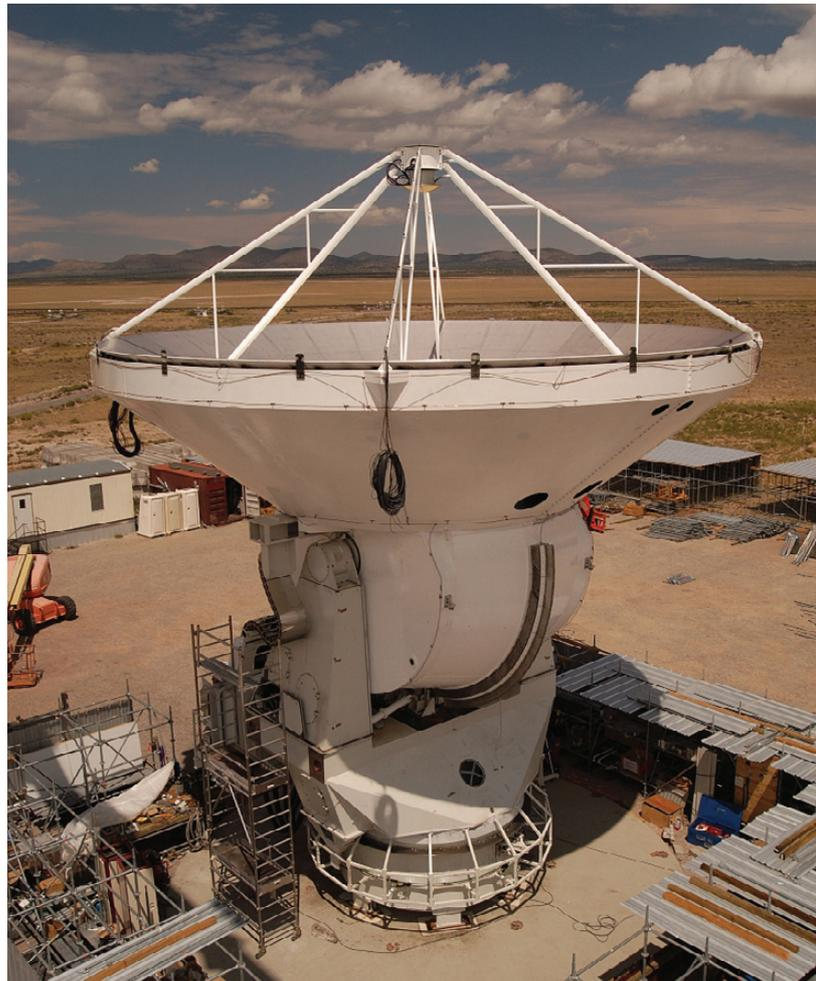
*The ALCATEL/EIE antenna in the final phase of assembly at the ATF.*
