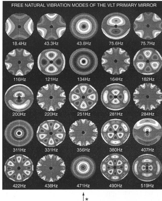
**Figure 5:** The first 25 natural vibration modes of the VLT primary. The first 16 of these are corrected by the active optics system. The modes shown were calculated for a thickness of 200 mm, whereas the final thickness of the mirror is 175 mm (W99).
