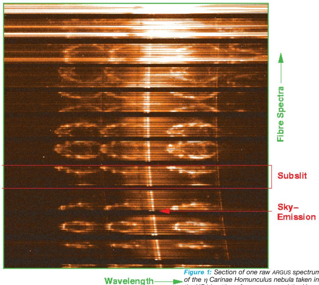
Figure 1: Section of one raw ARGUS spectrum of the  $\eta$  Carinae Homunculus nebula taken in the HR14 setting of GIRAFFE around the H $\alpha$  and the [NII] nebular emission lines.
