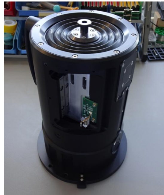
Position actuators: 792x3 Range 10mm, resolution 0.1nm BDC motor + piezo actuator
