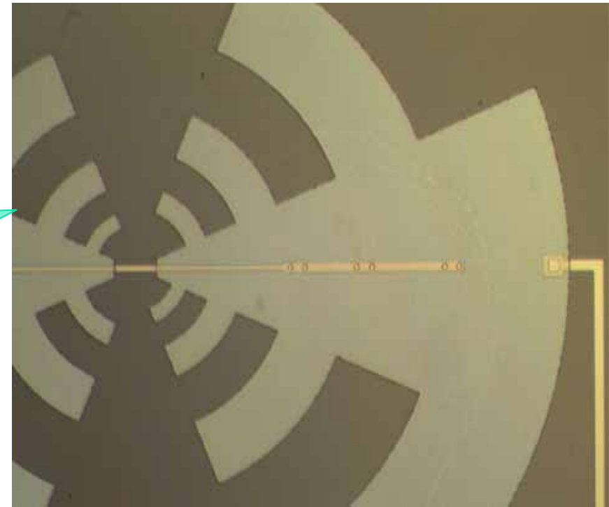
Distributed Junctions and log-periodic antenna
