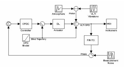
Figure 1: Schematic Layout of the Fringe Tracking Facility using FINITO
