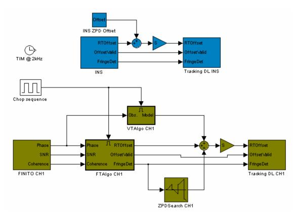
Figure 3: TAC Algorithm Schematic (1 DL, 1 FTK channel only)
