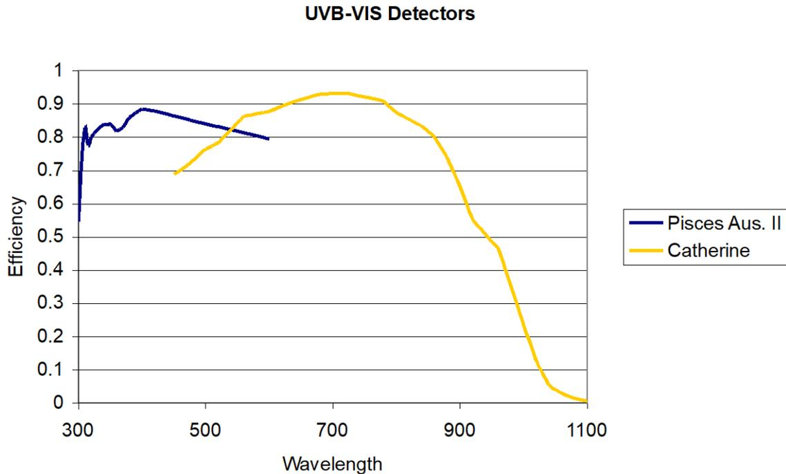
Figure 8: UVB/VIS detector efficiency.
