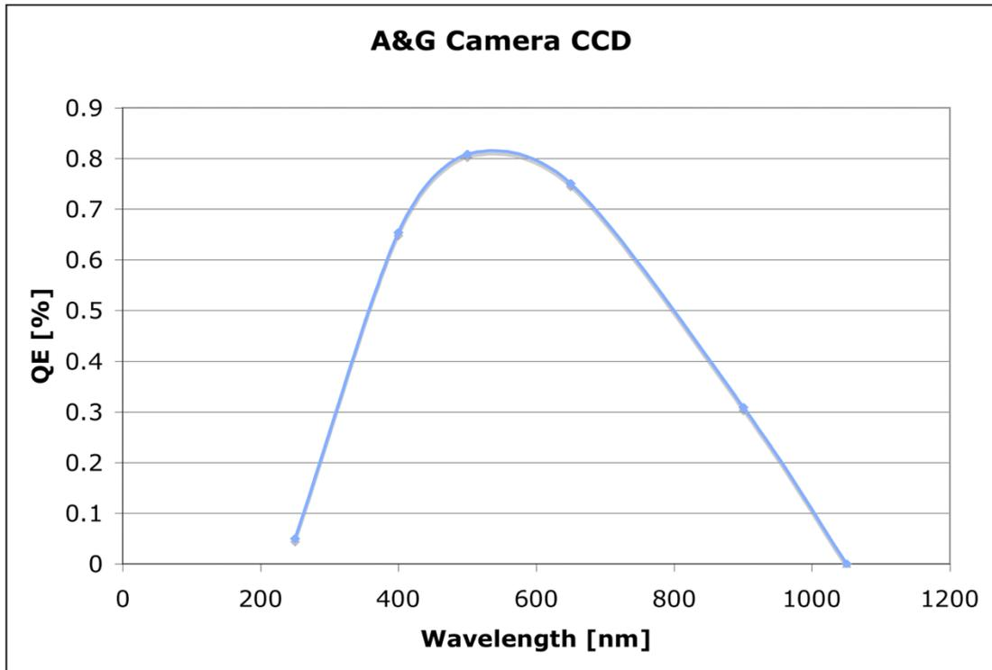
Figure 26: A&G TCCD quantum efficiency curve.
