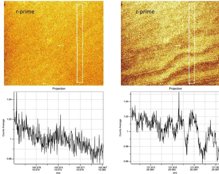
Figure 30: Fringing in r\_prime and z\_prime. The most affected filters are r\_prime, i\_prime, z\_prime, and I. The peak-to-peak amplitudes range from 2% in r\_prime to 4% in z\_prime.
