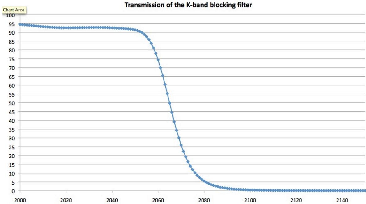
Figure 10: Transmission curve of the K-band blocking filter.
