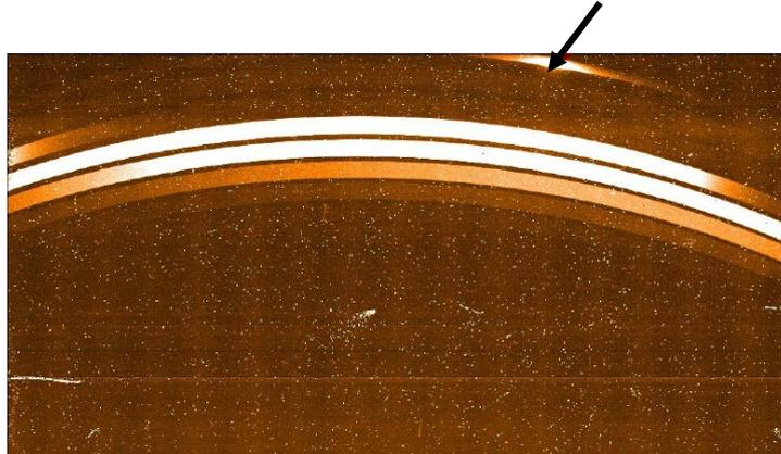
Figure 20: Leak in the K-band blocking filters.
