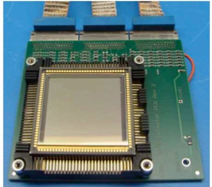
Figure 10: Left panel shows the AQUARIUS multiplexing readout scheme. Right panel shows the detector mounted in its socket.
