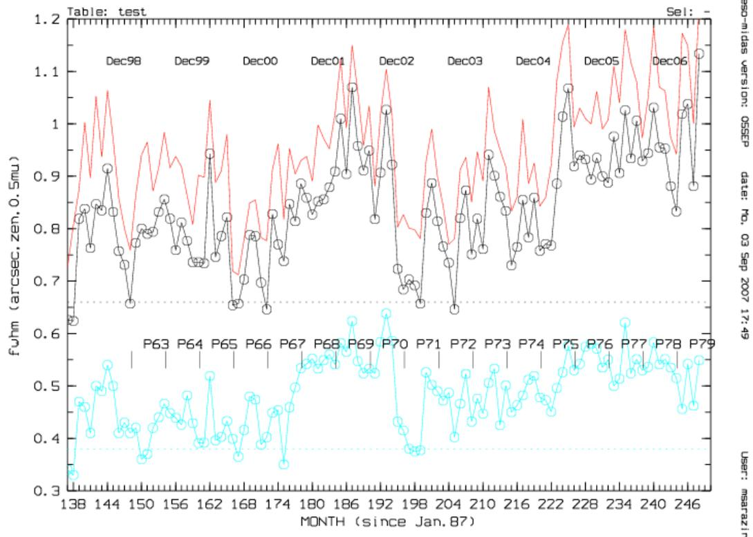
Figure 1: Statistical seeing distribution at Paranal since UT1 First Light. From top: monthly average (red, no symbol), monthly median (black, circles), 1989-1995 median=0.66" (dashed black line), monthly 5 percentile (blue, circles), 1989-1995 5 percentile=0.38" (dashed blue line). See text.
