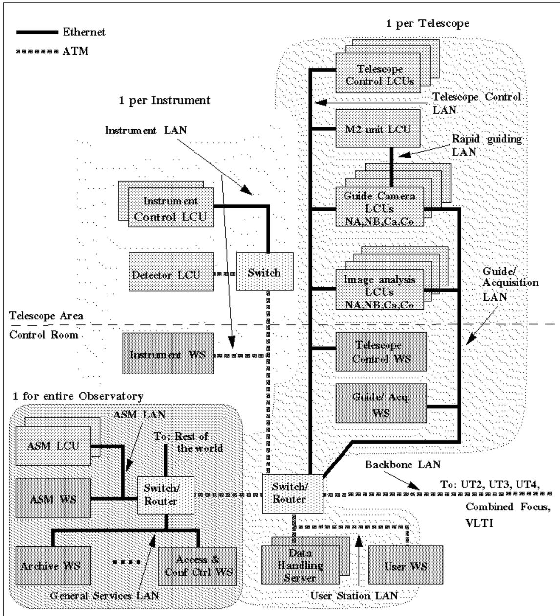
Figure 8: Logical lay-out of the VLT LANs
