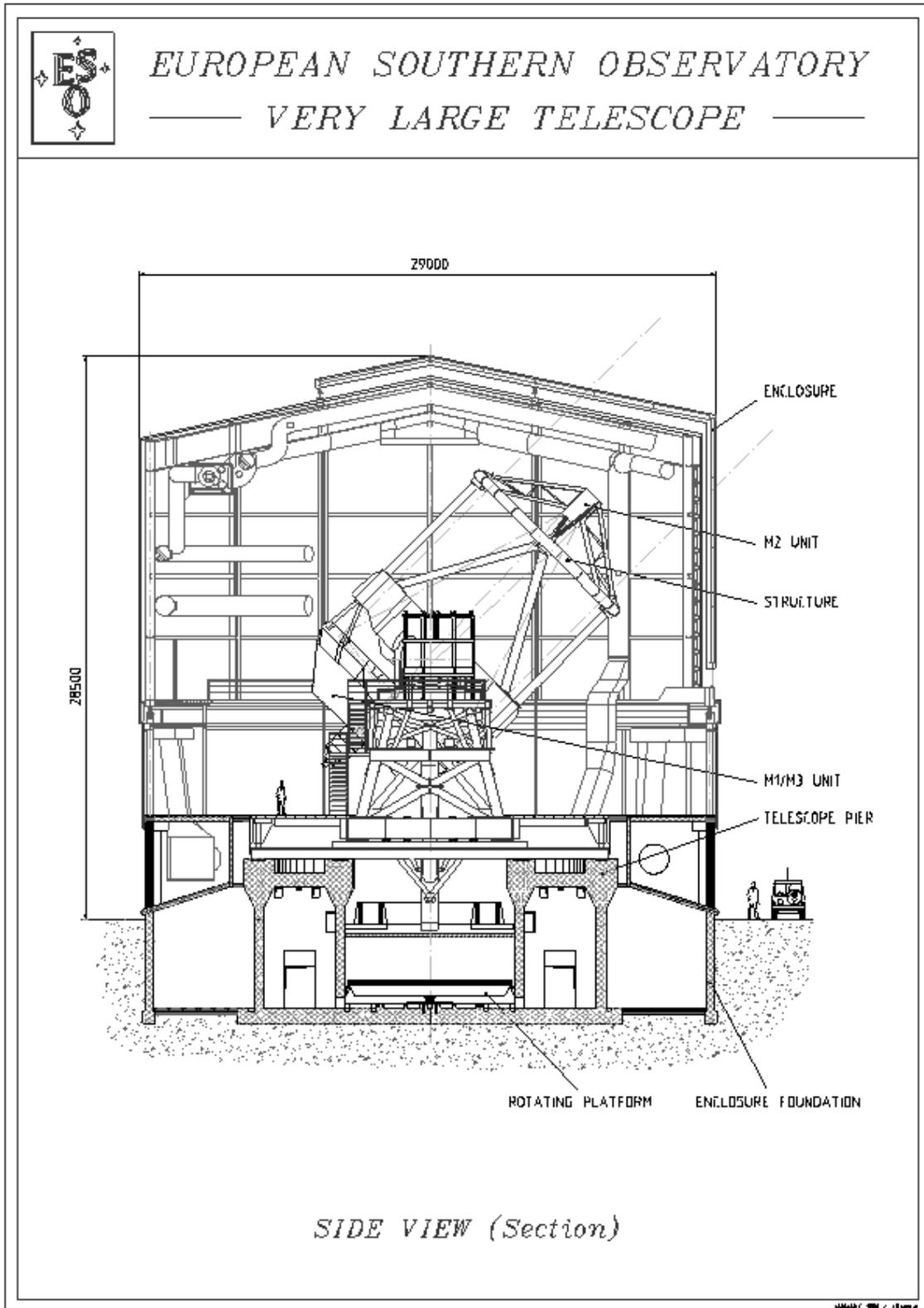
Figure 4: Side view of a Unit Telescope
