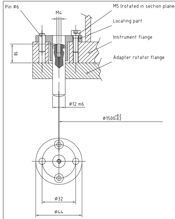
Figure 9: Proposed design for a reference pin adjustment device
