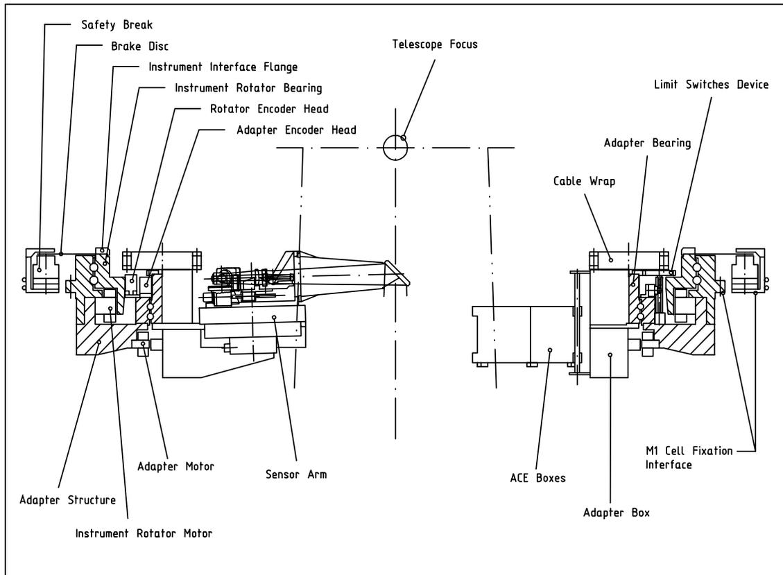
Figure 5: Cross section of the Cassegrain adapter/rotator. Note that in this view the light from the telescope comes from below. The design principles of the Nasmyth adapter/rotator are the same, the dimensions differ.
