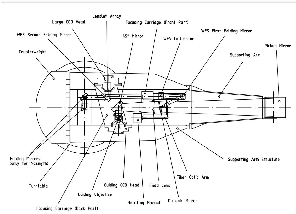
Figure 6: Schematic view of the adapter sensor arm.
