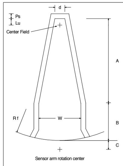
Figure 7: Guide-probe shadow in the Nasmyth focal plane. See table 4 for the dimensions.
