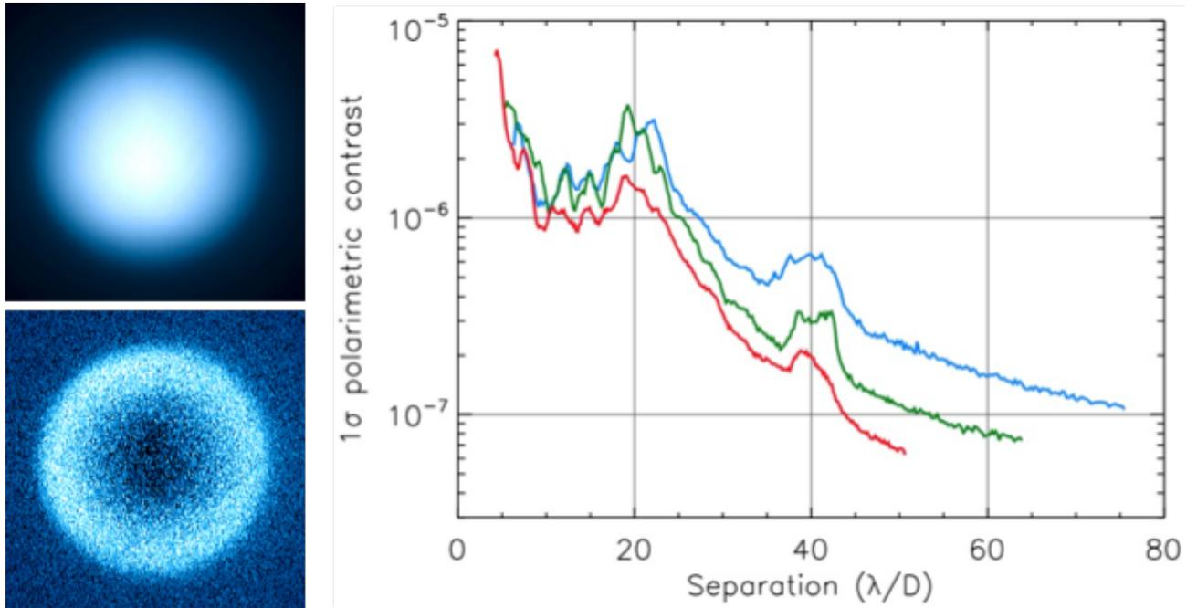
Figure 20: Top left: intensity image of Titan. Bottom Left: polarized intensity. Right: polarimetric contrast (right) on a bright target for the V (blue), N\_R (green), N\_I (red) filters.
