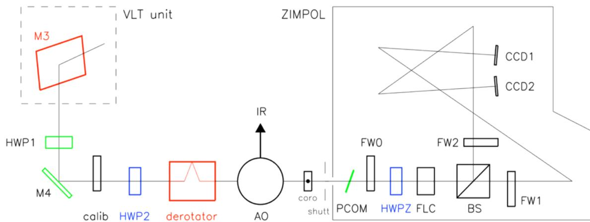
Figure 9: ZIMPOL optical path. Components, which introduce (red) or compensate (green) instrumental polarization, and those, which rotate the Stokes vector into the derotator system (blue), or instrument system (black) are indicated.
