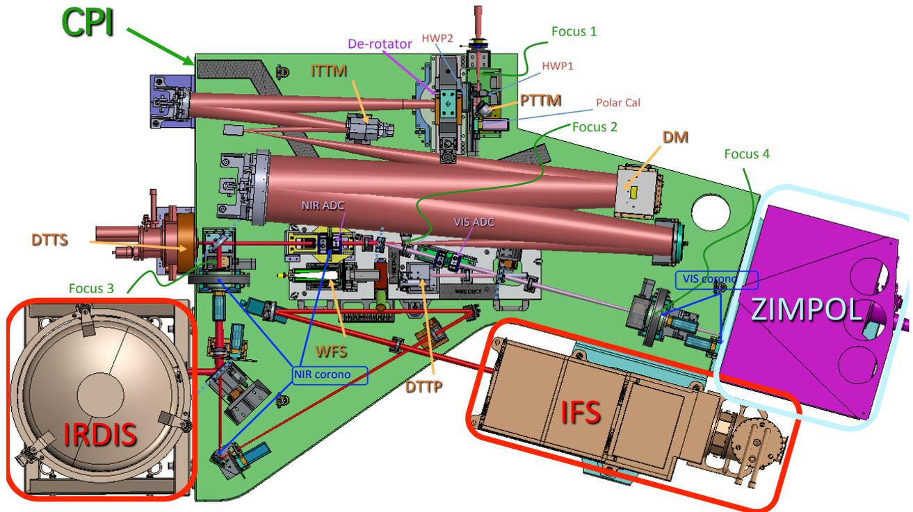
Figure 3: CPI, the common path optical beam on the main optical bench (green) feeding the 3 other sub-systems ZIMPOL (magenta), IRDIS (gray) and IFS (brown).
