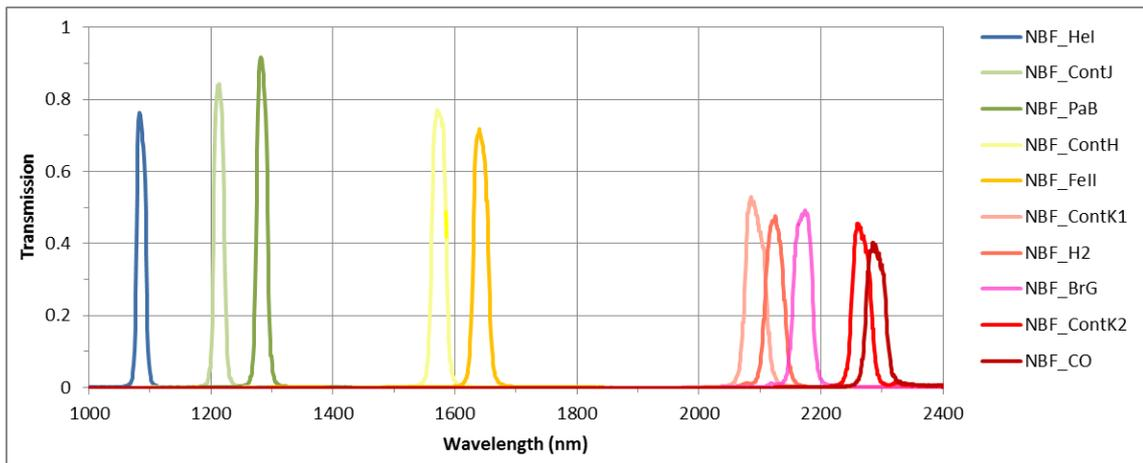
Figure 31: IRDIS NB filters.
