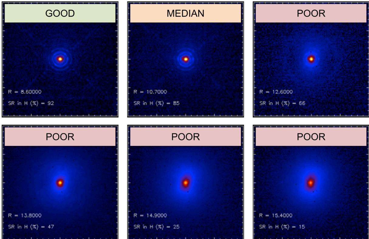
Figure 11: SPHERE PSF morphology and Strehl ratio as a function of R magnitude (see Table 997 and Table 10108 for details).
