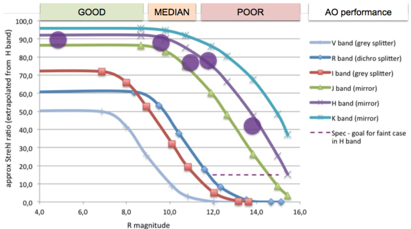
Figure 10: Theoretical and measured (purple circles) SPHERE-SAXO Strehl ratio as a function of R magnitude for good seeing conditions and different wavelength ranges from V to K (see Table 997 and Table 10108 for details).
