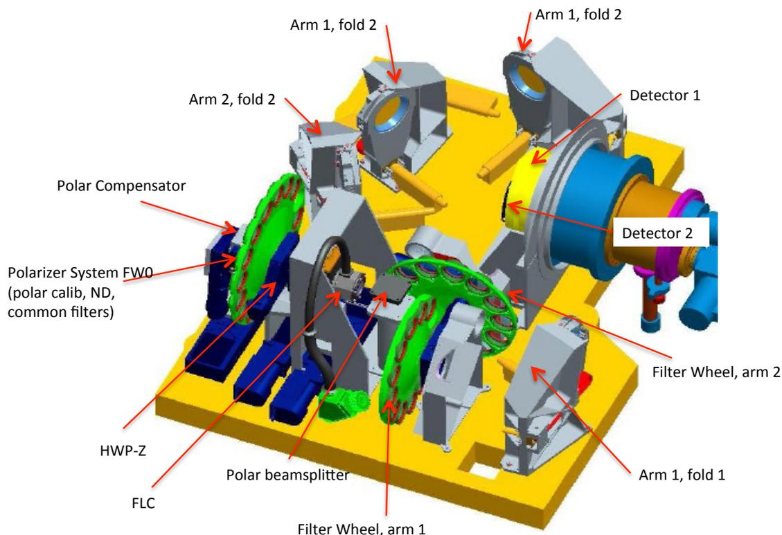
Figure 7: ZIMPOL schematic view showing the main elements of this visible polarimeter, from polarization compensator, common filter wheel, Ferroelectric Liquid Crystal (FLC) modulator to the splitter, filter wheels 1 and 2, and the two detectors.
