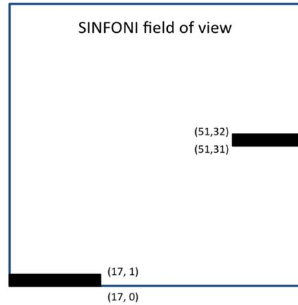
Fig. 2: Left: Appearance of the “blind spot” on the SINFONI detector. Right: The location of the blind spot with respect to the FOV.
