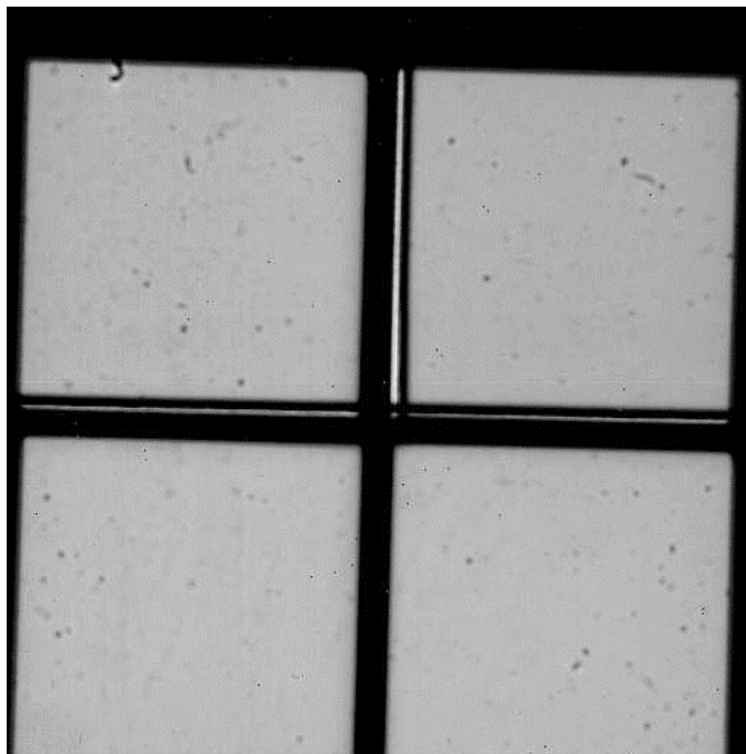
Figure 5-3: Flat field image of the SDI+ mode. The transmitted wavelengths are 1.6 mm (top left), 1.575 mm (top right) and 1.625 mm (bottom left and right).
