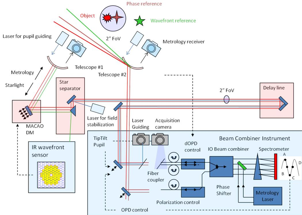
Figure 3: Working principle of GRAVITY with UTs.
