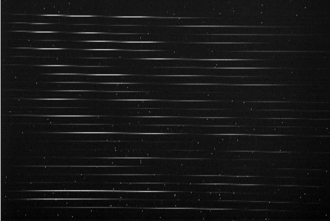
Figure 1: One raw GRAVITY frame of the science channel. Wavelength runs horizontally. In contrast to other beam combiners, GRAVITY does not record entire fringe packets but only four points on the central fringe (i.e. the so-called ABCD method of fringe detection). For each polarisation, each pair of telescopes yields thus 4 spectra. The fringe can be seen by comparing spectra pertaining to the same pair of telescopes. The total number of spectra is thus 24: 6 pairs of telescopes, 4 points ( viz. A, B, C, D) per pair.
