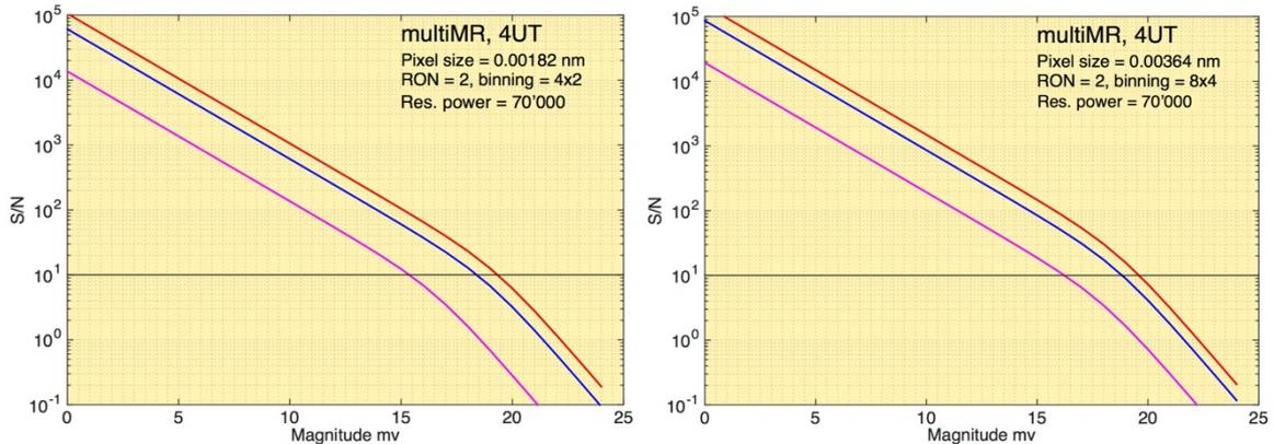
**Fig. 15: Left: S/N vs. stellar magnitude obtained in the multiMR42 mode for exposure times of 60s (pink), 1200s (blue) and 3600s (red). The slope change defines the magnitude at which the measurement becomes detector read-out noise limited. Right: same but for the multiMR84 mode.**
