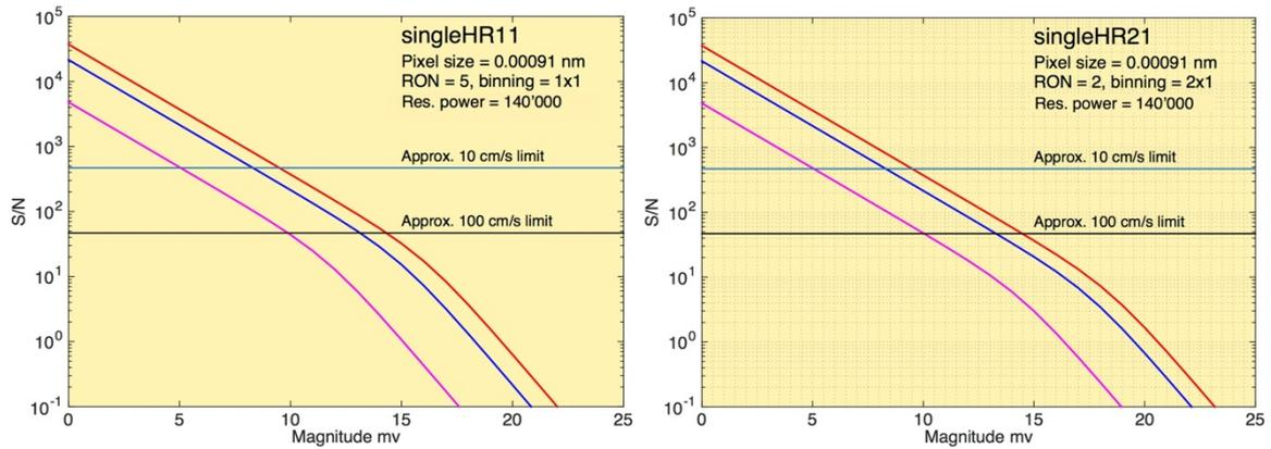
**Fig. 13: Left: S/N vs. stellar magnitude obtained in the singleHR11 mode for exposure times of 60s (pink), 1200s (blue) and 3600s (red). The slope change defines the magnitude at which the measurement becomes detector read-out noise limited. S/N for 10 cm s<sup>-1</sup> and 100 cm s<sup>-1</sup> are shown. The values are rough estimates for slowly-rotating, inactive late-G or K dwarf stars, calculated for a seeing of 0.8 arcsec and an airmass of 1. Right: same but for the singleHR21 mode.**
