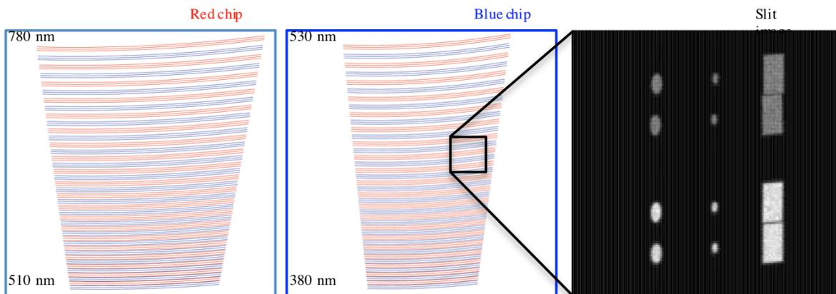
**Fig. 6: Format of the red spectrum. Left and centre: format of the blue spectrum. Right: Zoom in on the pseudo-slit image. The latter shows the image of the target (bottom) and sky fibre (top). Each fibre is re-imaged into two slices. The image of the pseudo-slit on the science detectors, from left to right: in the 1-UT UT mode, in the 1-UT UHR mode, and in the 4-UT MR mode, are shown together.**
