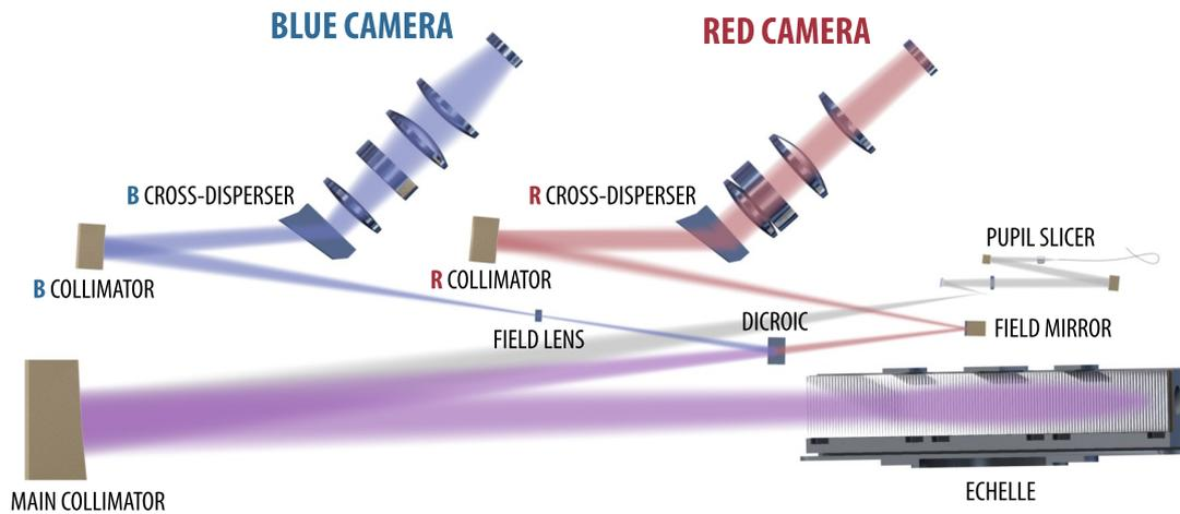
**Fig. 4: Schematical layout of the ESPRESSO spectrograph and its optical elements.**
