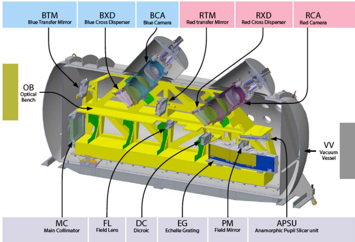
**Fig. 7: Opto-mechanics of the ESPRESSO spectrograph.**
