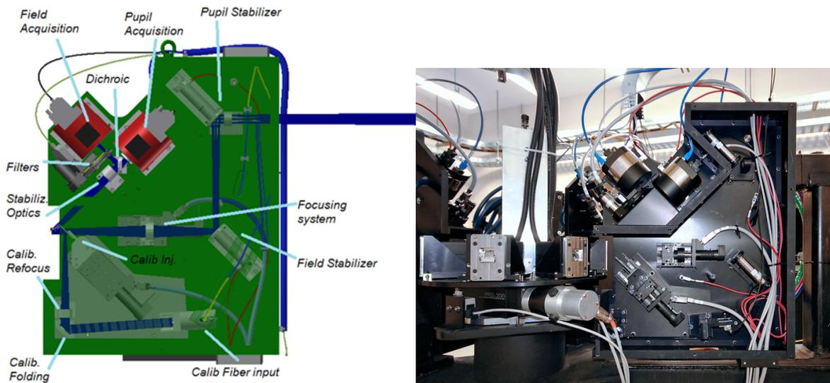
**Fig. 2: Side view of an individual Front-End Unit.**
