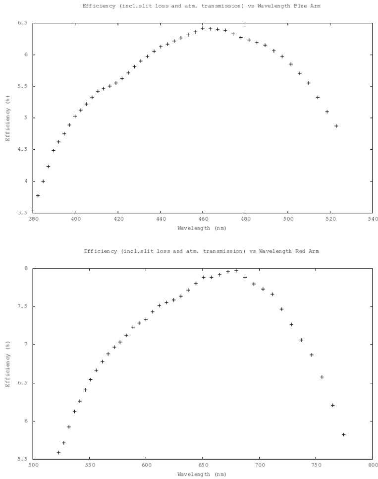
**Fig. 11: Total transmission of ESPRESSO incl. slit losses and atmospheric transmission in HR (and MR) mode for the blue (top) and red arm (bottom). A seeing of 0.8 arcsec and an airmass of 1 are assumed.**
