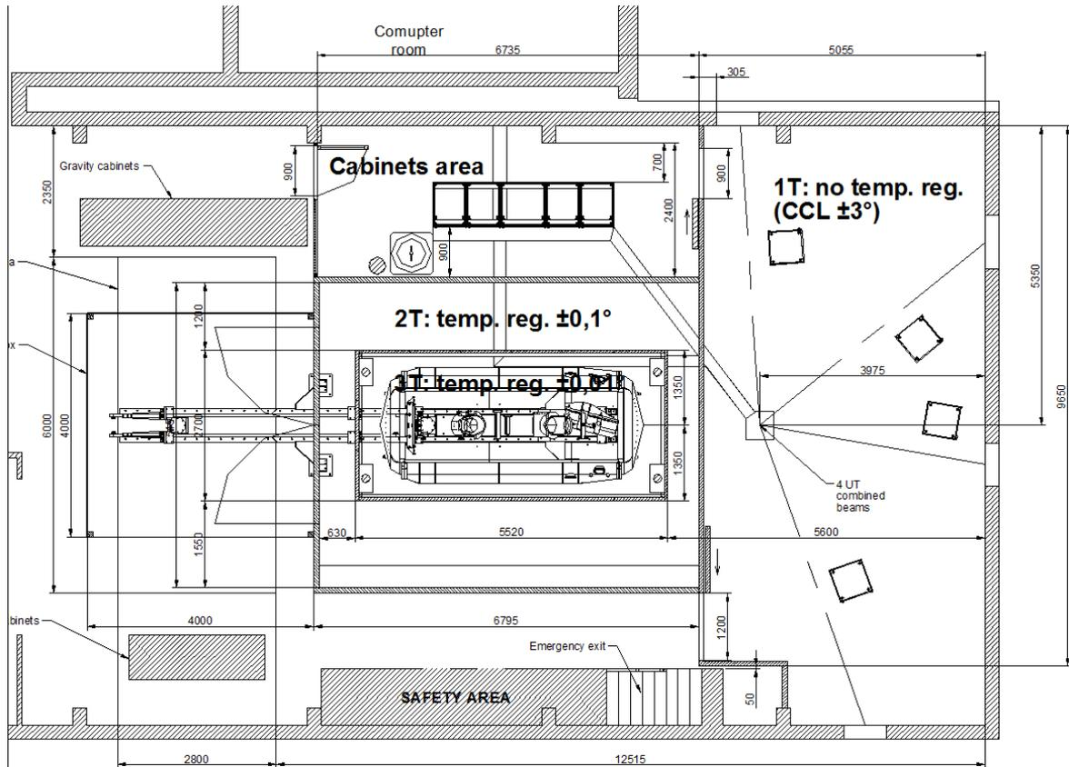
**Fig. 9: Schematic diagram of ESPRESSO inside the CCL, top view.**
