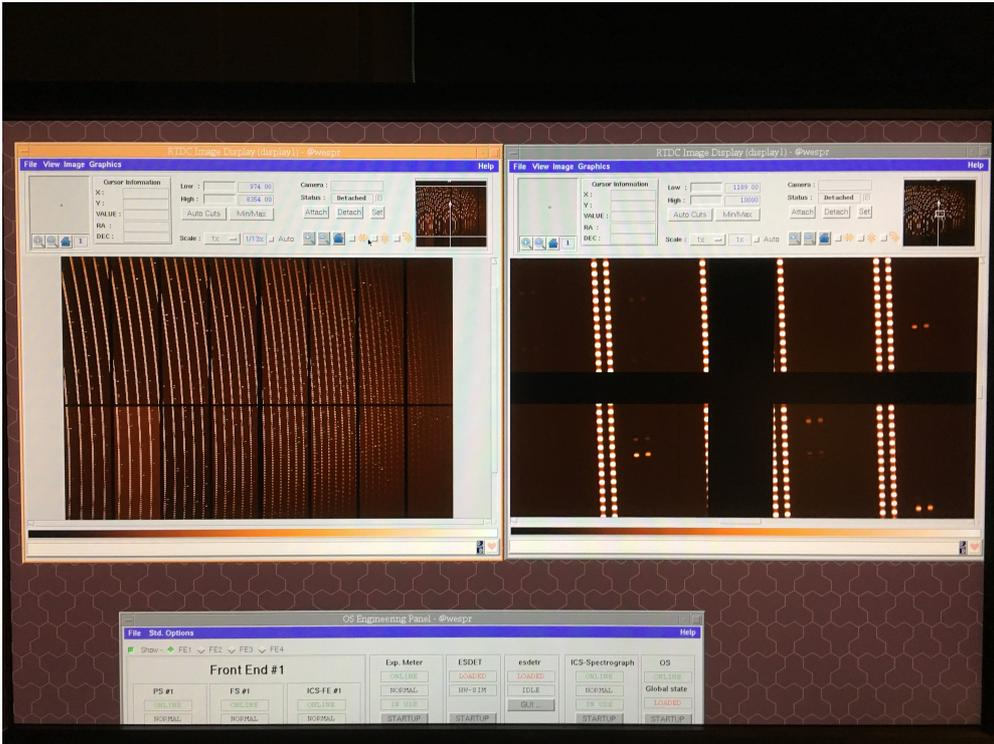
**Fig. 16: Example of raw frame plus zoom in, on the right-hand side, from the red CCD of ESPRESSO illuminated with the ThAr lamp (in Fibre A – to the right) and the Fabry-Pérot simultaneous calibration light (Fibre B; continuous dots to the left)**
