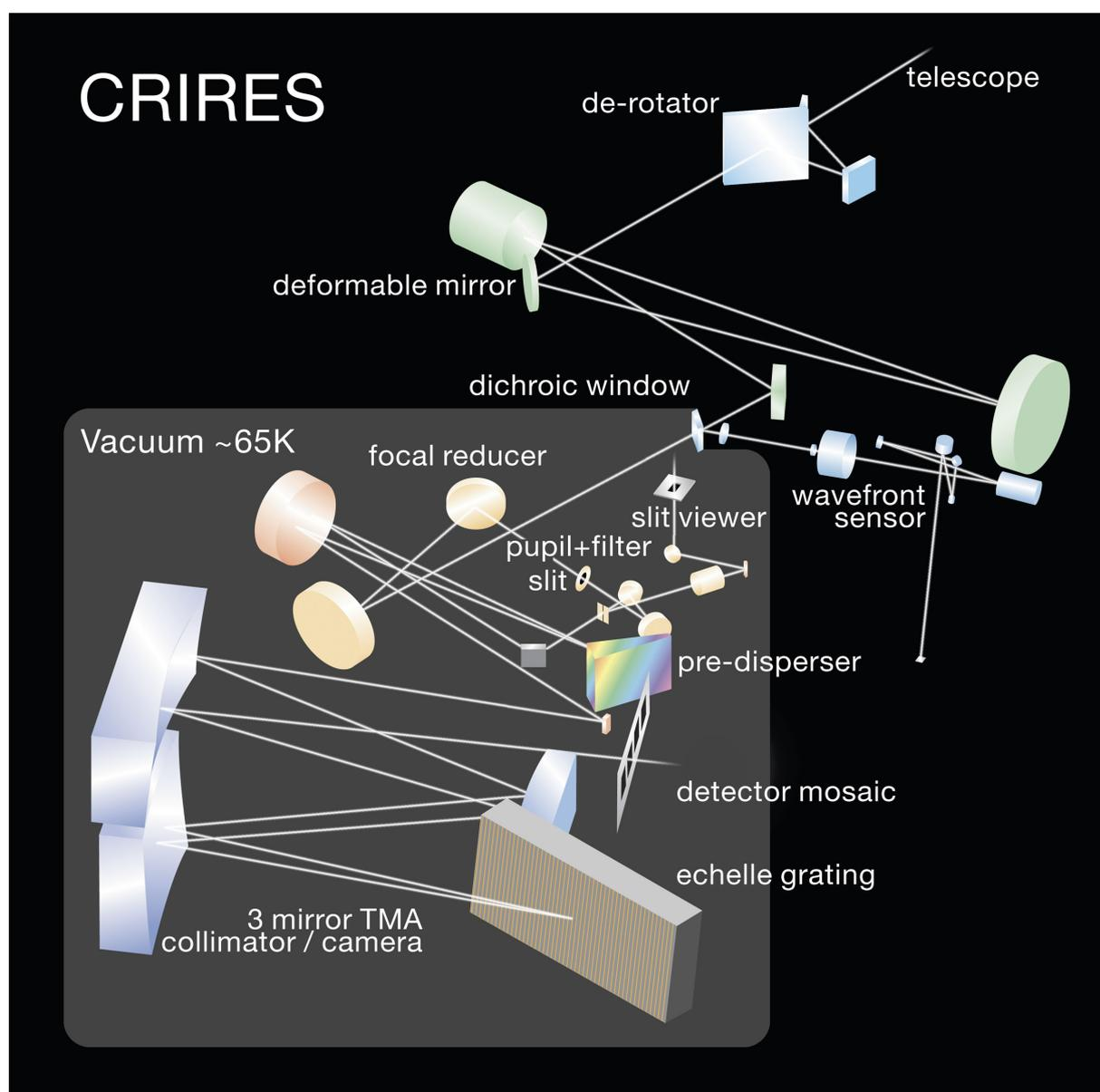
Figure 1: Layout of the CRIRES optical design.
