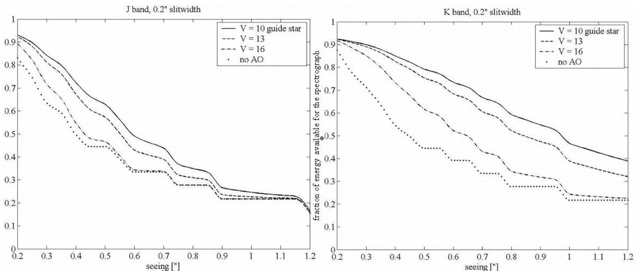
Figure 10: The fraction of energy available for the spectrograph in a  $0.2''$  slit, as a function of optical seeing is shown for the J (left) and K (right) band for AO stars of  $V=10, 12, 16$  mag and without AO correction. For reference please consult the [Exposure Time Calculator, \(ETC\)](#).
