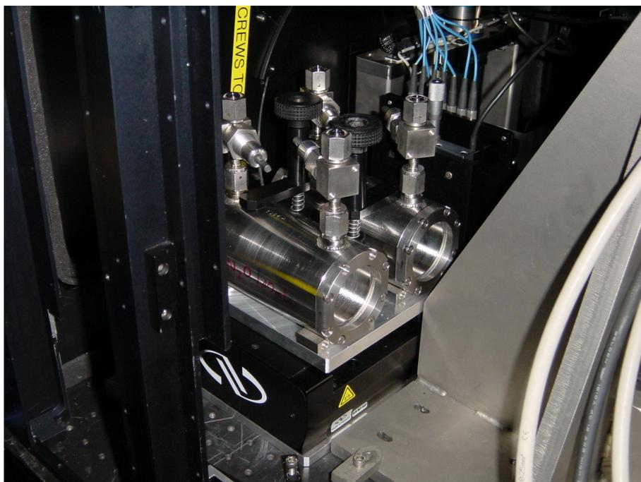
Figure 16: The N<sub>2</sub>O and CO gas-cells mounted on the carriage
