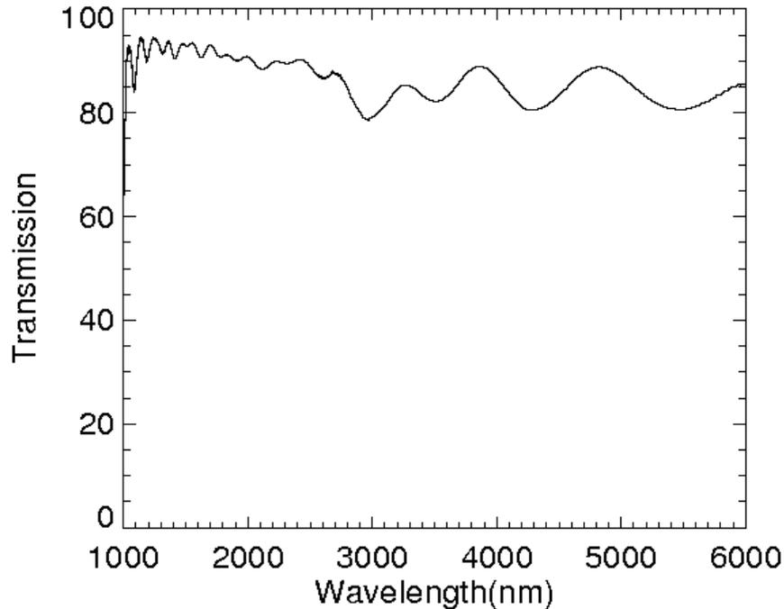
Figure 21: Transmission curve of the entrance window.
