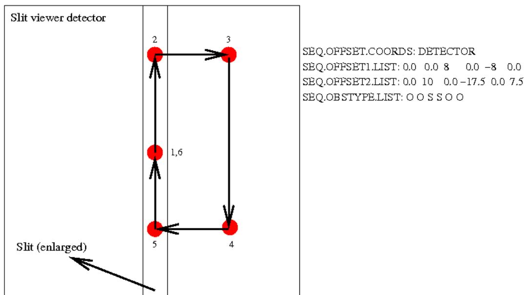
Figure 28: Illustration showing the apparent locations of a target as seen on the slit viewer detector for the given parameters, in the case of 'DETECTOR' coordinate offsets. Although the derotator mode must be set to 'SKY', the position angle is irrelevant since all the motions are made in detector coordinates.
