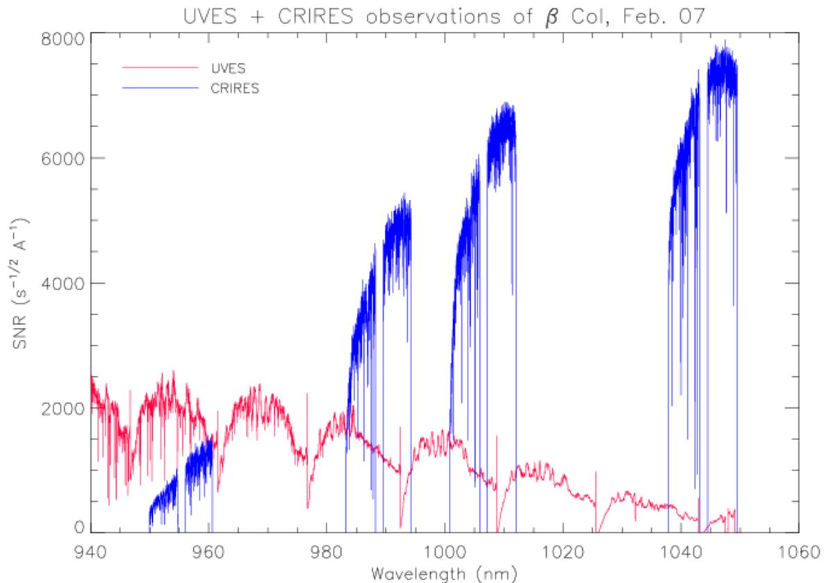
Figure 22: Comparison of  $S/N/\text{\AA}$  per second $^{1/2}$  of integration time obtained during nearly simultaneous CRIRES and UVES observations of  $\beta$  Col. Courtesy S. Uttenthaler. New observations are planned to compare the two systems after the UVES red CCD upgrade in July 2009.
