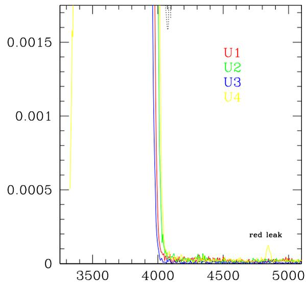
Figure 4: Detection of a very small “red leak” in the U-band efficiency curve of Q4. Note that the y-axis has been zoomed in by a factor of 200 compared to Fig. 3. The peak of the red leak is about 0.1% of the efficiency peak.
