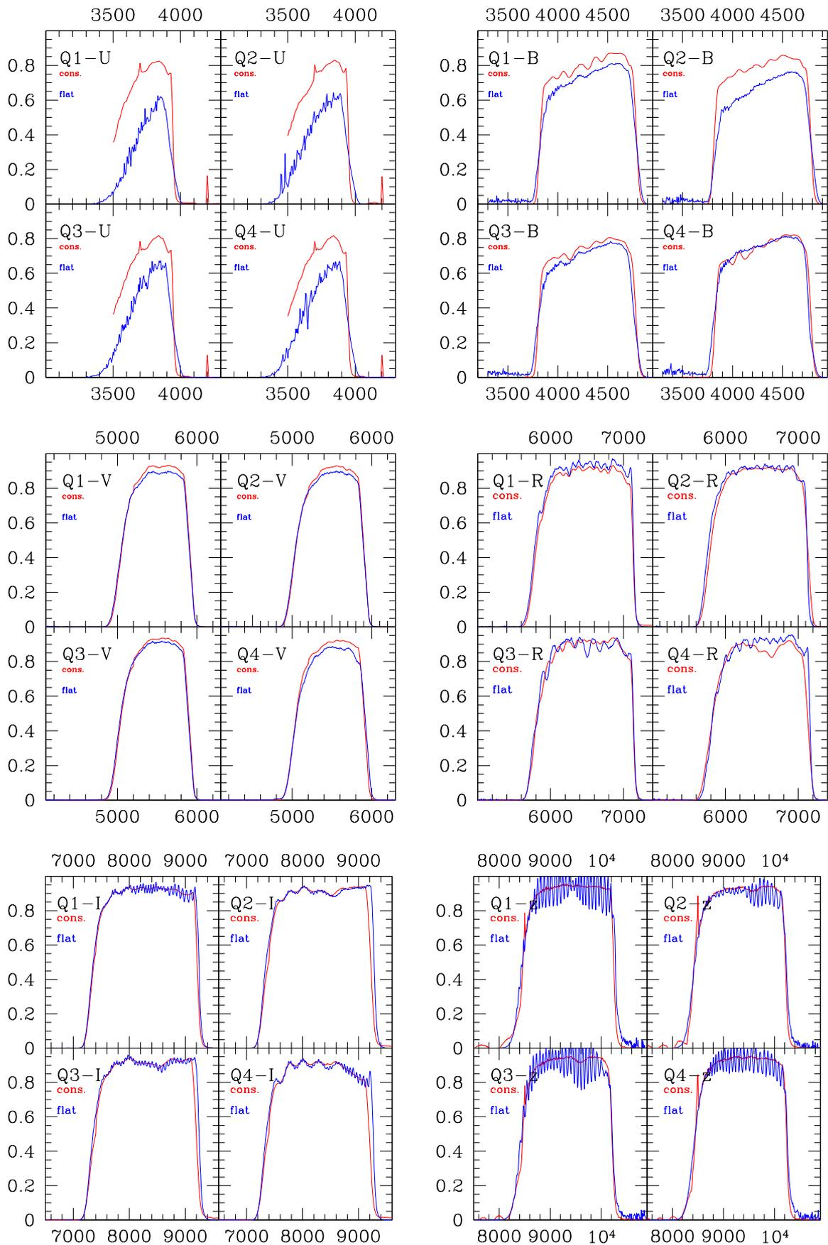
Figure 2: . Filter transmission profiles for VIMOS UBVRIZ. X-axis is in units of Å.
