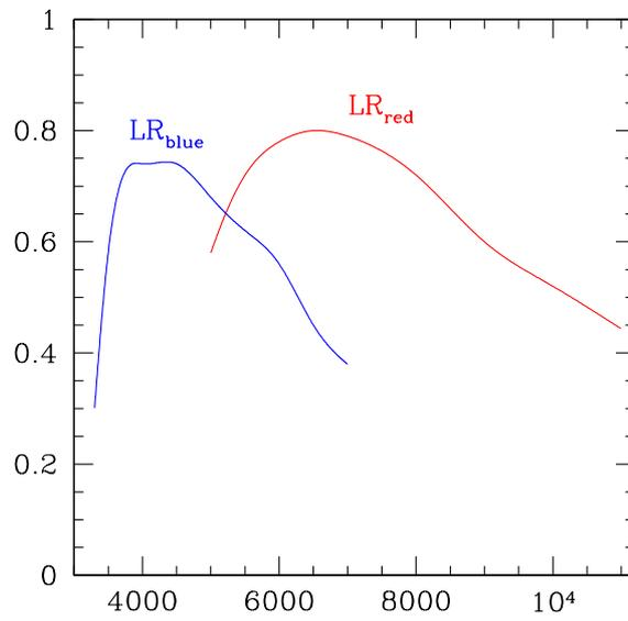
Figure 1: Consortium transmission profiles of the LR red and blue grism. X-axis is in units of  $\text{\AA}$ .
