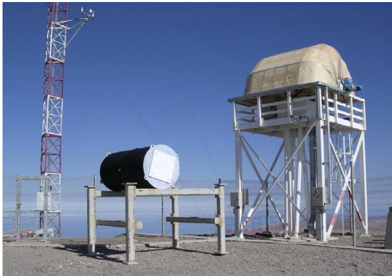
Figure 5-17: Steel pipe exposed to sun radiation
