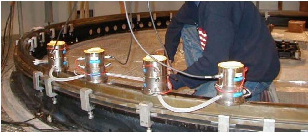
Figure 9-37: Communicating vessels measurement
