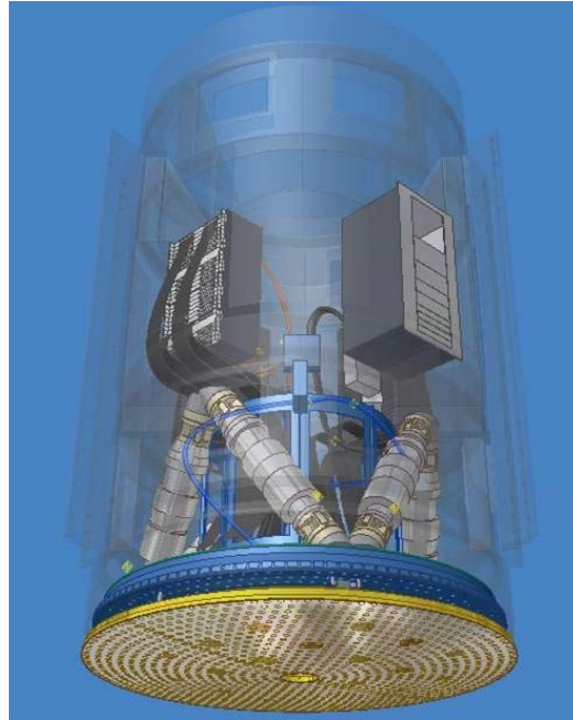
Figure 8-28: Conceptual design for the 1120mm diameter, 1170 actuators VLT deformable secondary mirror.
