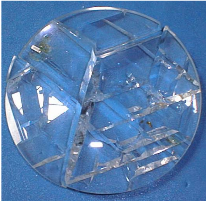
Figure 14: The lens brakes during a cooling in 40 mn
