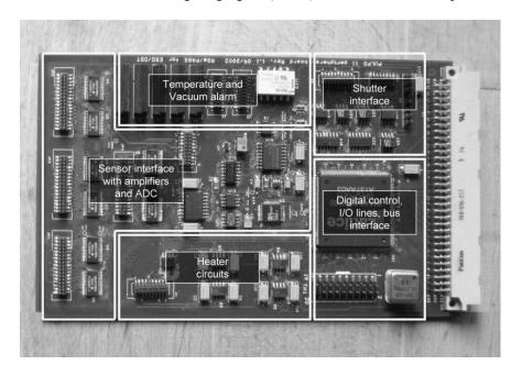
Figure 3. PULPO 2 Peripheral Board
