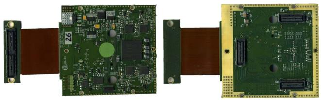
**Figure 9:** AD board top. The board is connected to the Main board via a flex PCB.
