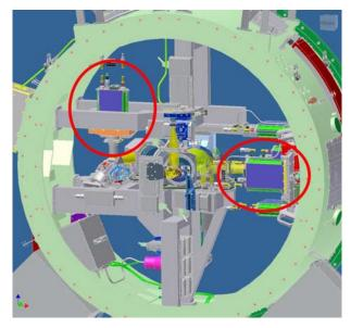
**Figure 28:** GALACSI with two of the four AO cameras highlighted. (Tip/tilt camera not visible)
