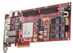
Figure 14: COTS PCI-e board on the back-end PC Linux computer.
