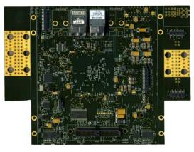
**Figure 6:** AONGC Main board bottom. On the upper side of the board one can see the low-profile optical transceivers LNP-LT12HB (1320nm) and LNP2-ST11HB (850nm), see reference [6].
