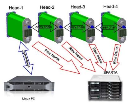
Figure 2: Multi-head connection architecture.
