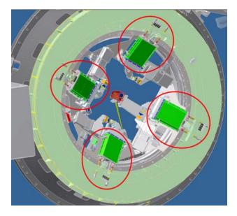
**Figure 27:** ESO AOWFS cameras on GRAAL. Two additional ones (Tip/tilt and MCM camera) are not visible.
