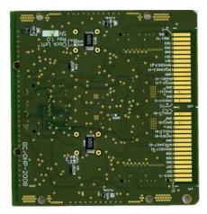
**Figure 12:** Clock board bottom. On the left side one can see the pads for the spring contacts that connect to the CCD.
