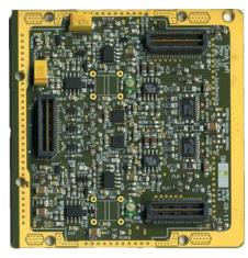
**Figure 11:** Clock board top. The three connectors interface this board to the AD board.
