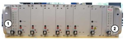
Figure 19: Rear side of the power supply showing the voltage supervisors on either side, one for the front set of power supplies *1*), and the other for the rear *2*).
