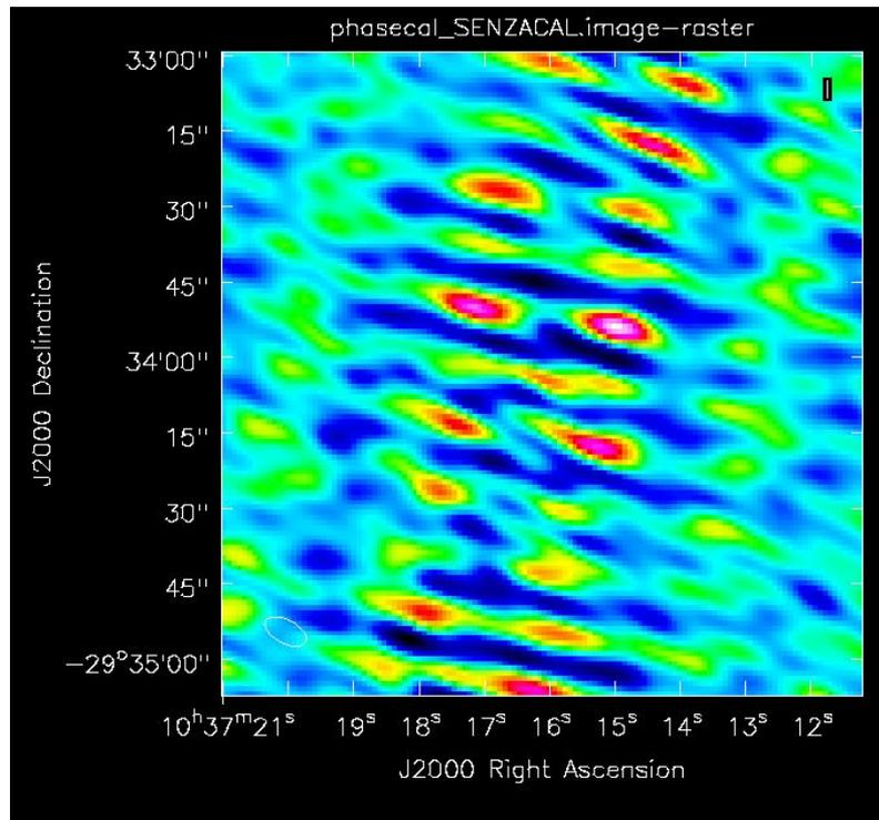
The Fourier transform of raw visibilities of a point source
