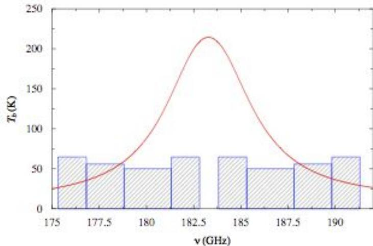
Four “channels” flanking the peak of the 183 GHz water line
