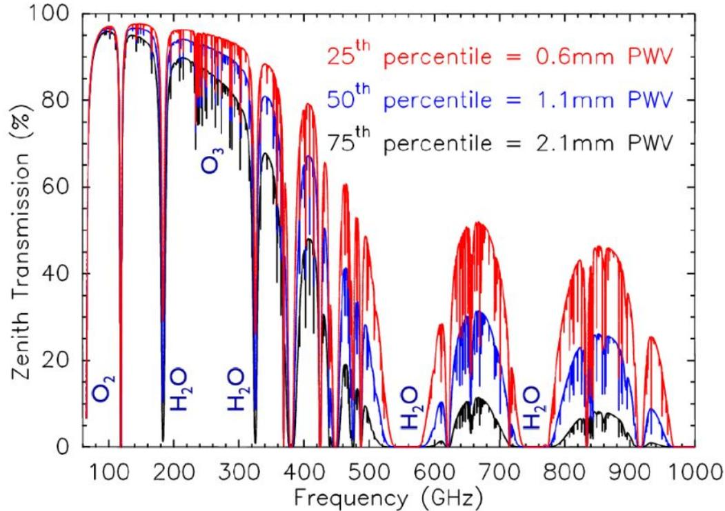
The transmission curve changes with Precipitable Water Vapor content in the atmosphere!
