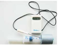
Measuring the temperature at the start of the reaction
