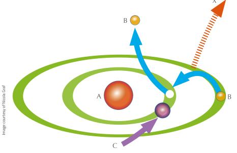
PIXE: an inner-shell electron is removed by a particle beam and the vacancy left behind is filled by an electron from an outer shell, giving rise to the emission of characteristic X-rays. A: atomic nucleus; B: electron; C: particle beam; X: characteristic X-ray emission
