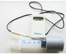
Measuring the temperature during the reaction
