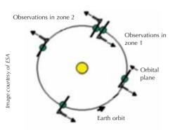
CoRoT is pointed in the same direction for more than 150 days at a time, before the Earth's movement around the Sun leads to the unwanted effect of the Sun's rays entering the telescope. CoRoT then turns 180 degrees around its long axis and points in the other direction
