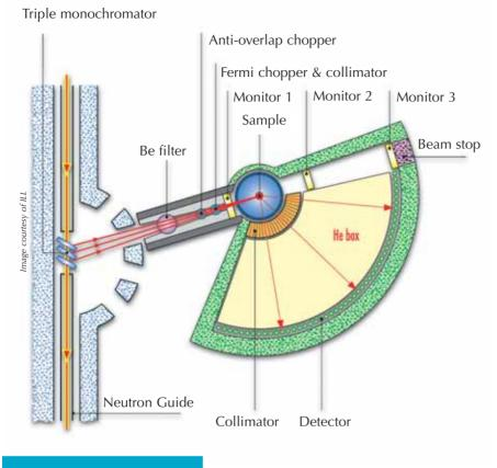
The layout of the IN6 neutron scattering spectrometer at ILL
