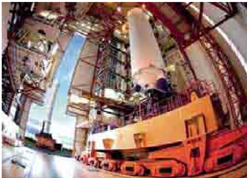
Solid rocket booster arrives for integration with the main cryogenic stage for Jules Verne's Ariane 5 ES launch vehicle
