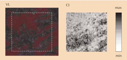
Visible light (VL) microscopy image and atomic distribution of chlorine of one of the samples with moderate alterations (obtained by micro X-ray fluorescence with an exciting beam of 3.9 keV)
