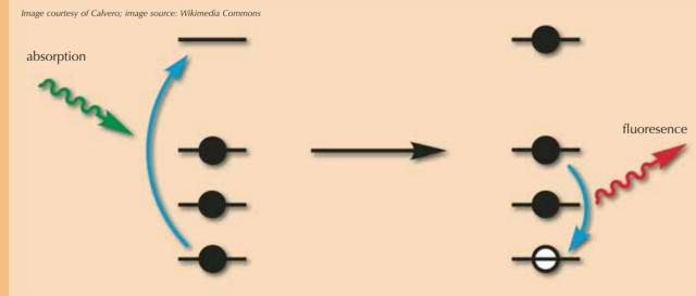
Electrons absorb X-ray light and move to a higher energy level (left). When electrons move to a lower energy level, they release energy in the form of fluorescence (right)
