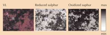
Normalised images of the distribution of the reduced (intact) and oxidised (altered) sulphurs on the most degraded sample (8 x 7 mm<sup>2</sup>)
