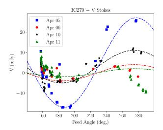
Figure 21. Reconstructed Stokes V of 3C 279 as a function of feed angle,  $\phi$ , during the EHT campaign. Stokes V is computed as the real part of  $(XY^* - YX^*)/j$ . Dashed lines show the simplified model of Eq. G2, based on cross-polarization phase offset,  $\beta$ , of the APP reference antenna.
