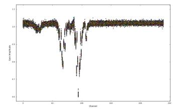
Figure 23. Bandpass for Sgr A\* core (after removing instrumental bandpass with the calibrator NRAO 530) for 2017 Apr 07 observations. Only baselines longer than 60-m were used to remove virtually all of the extended arcsecond emission. For each channel, every antenna bandpass amplitude is plotted (represented by different colors). All three April observations show virtually the same 'bandpass'.
