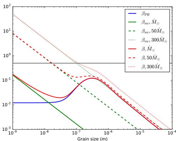
**Fig. 5.**  $\beta$  as a function of grain size. The material used for  $\beta_{PR}$  is M1 of Schüppler et al. (2015). Three hypotheses for the mass-loss rate of the star are shown (solid, dashed, and dotted lines). The horizontal solid black line is the upper limit for bound trajectories assuming zero eccentricity for the parent body, see Sezestre et al. (2017) for further details.
