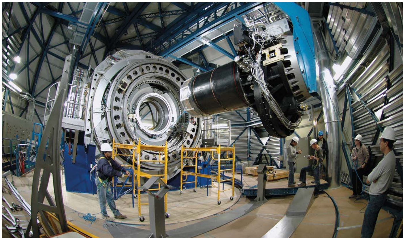
Figure 1. VIRCAM insertion into M1 of VISTA.
