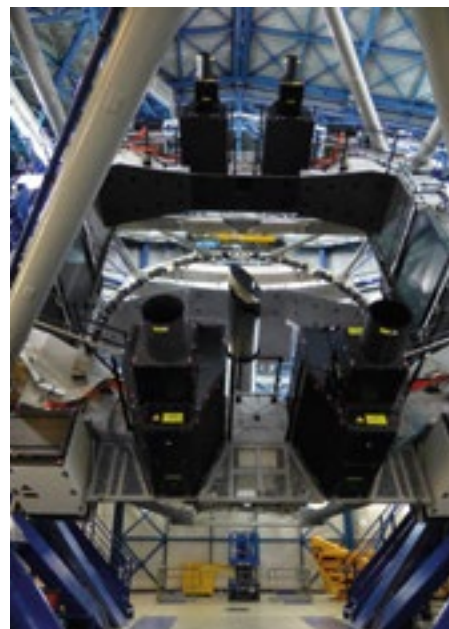
Figure 5. The four laser guide star units mounted on the UT4 centrepiece with their respective laser and instrument control cabinets.
