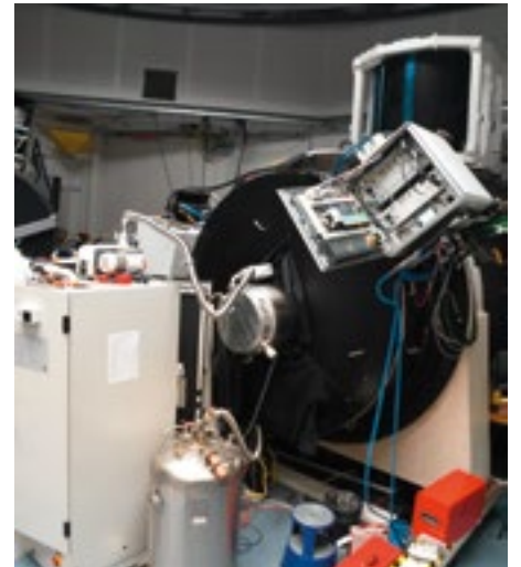
Figure 5. The AOF test configuration in the old integration laboratory in Garching. The DSM sits on top of the ASSIST bench and the GRAAL module is mounted on the Nasmyth focus simulator. In the foreground the CAMCAO silver cryostat can be seen; this camera is used to record output images corrected by the adaptive optics.
