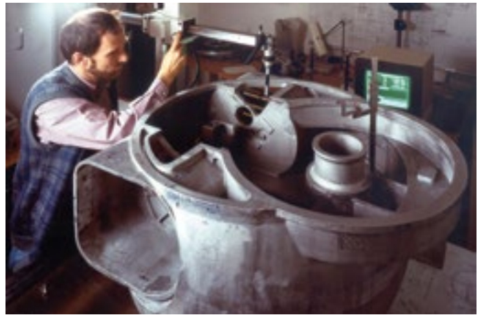
Figure 2. A younger Jean-Louis Lizon than in Figure 1 checks the ISAAC cold structure #1 during the construction phase in 1995.
