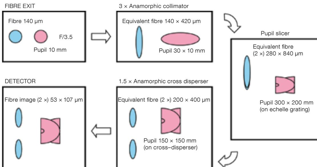
Figure 3. Conceptual description of pupil and fibre image at relevant locations of the ESPRESSO spectrograph.
