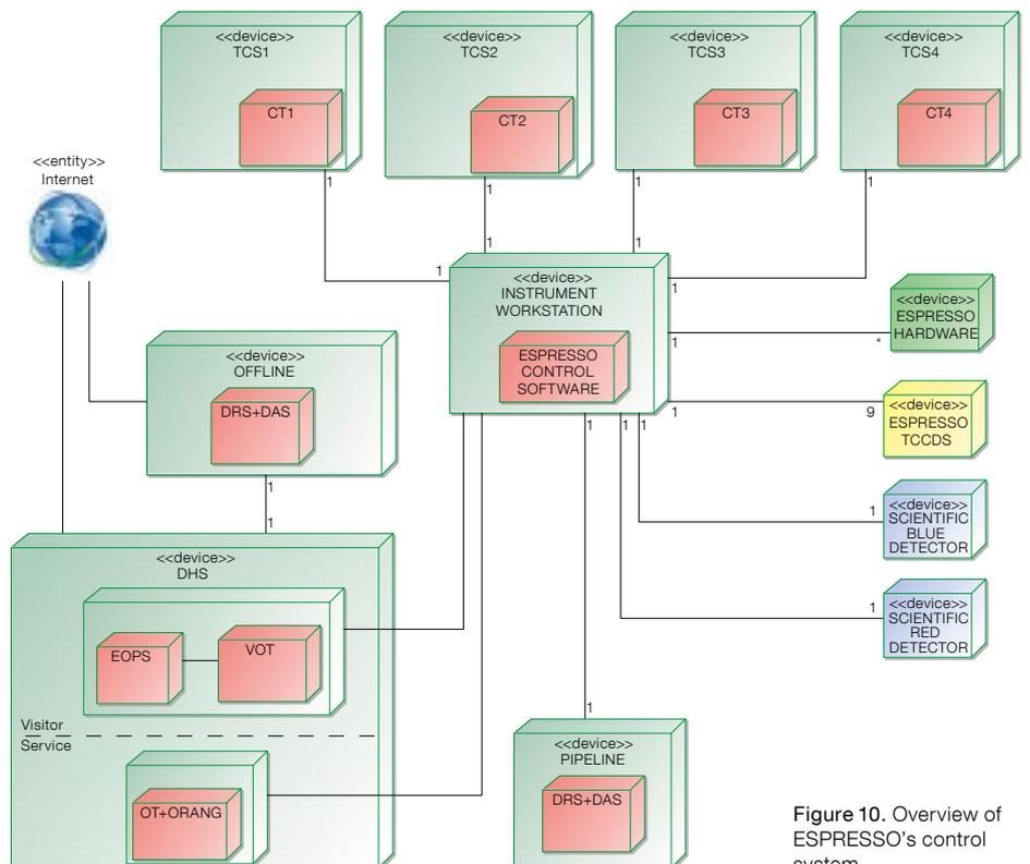
Figure 10. Overview of ESPRESSO's control system.
