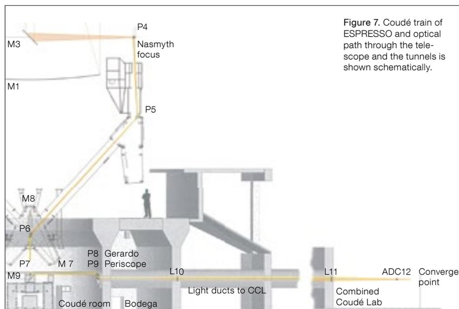
Figure 7. Coudé train of ESPRESSO and optical path through the telescope and the tunnels is shown schematically.
