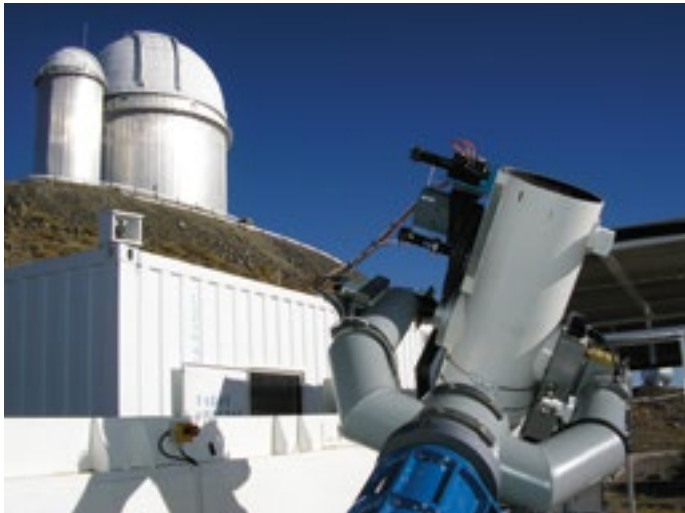
Figure 2. The TAROT La Silla telescope is located at the foot of the hill below the ESO 3.6-metre telescope in the former GMS building. Computers and electrical devices are stored in the adjacent shelter. The telescope does not require any human presence and observes every (clear) night.
