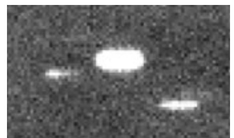
Figure 4. Trailed image of GRB 121024A. To obtain a time-resolved optical light curve during the first minute of the observation of a GRB, we trail the image such that each star occupies a small 10-pixel track on the frame. In this case TAROT observations started 45 seconds after Swift detected the event. The stars in the middle and right part of the image have a constant brightness during the exposure while the GRB optical counterpart is the left trail. At the start of the trail the brightness was R = 14.5 mag. At the end of the trail the magnitude had increased by 1.5 magnitudes only 60 seconds later! Just after this image, TAROT quickly provided the accurate position of the GRB allowing spectroscopy to be obtained with the VLT X-shooter spectrograph less than two hours later (Tanvir et al., GCNC 13890). The redshift of the source is 2.3, corresponding to an event that occurred 10.8 billion years ago.
