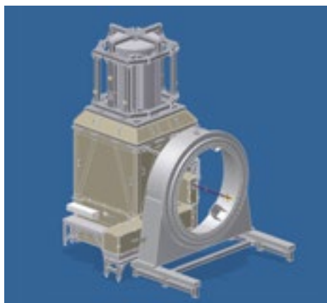
Figure 9. The ASSIST test bench (left) with the new generation M2 unit on top of the structure. The large 1.7-metre mirror is at the bottom (hidden by the light covers in this illustration) and the Nasmyth adaptor/rotator test bench can be seen on the right-hand side to allow the AO modules to be mounted. On the right is the secondary mirror (AM2), a 140 mm convex aspherical mirror manufactured by ASTRON, that completes the main tower optics of ASSIST.
