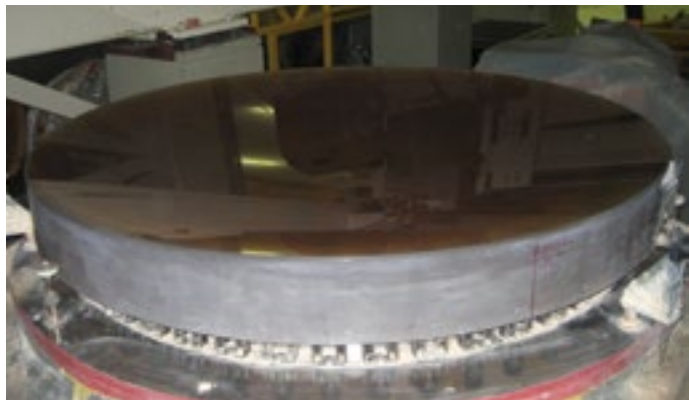
Figure 10. The main 1.7-metre mirror of ASSIST is shown at AMOS in Belgium during the last step of aspherical polishing.
