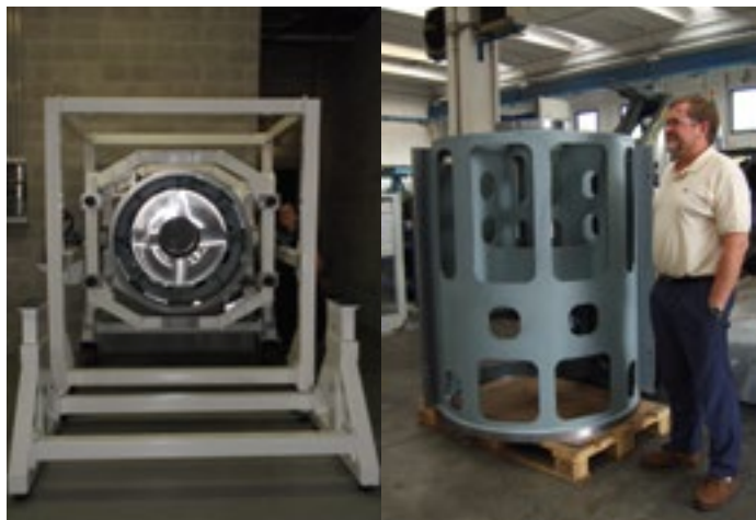
Figure 5. Integration and service stand for the DSM. The M2 hub, including the DSM, is mounted inside.
