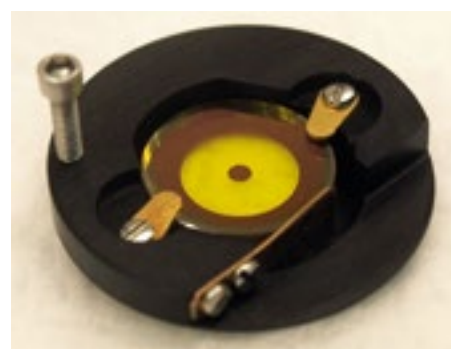
Figure 4. The APP optical element prior to installation in CONICA. The light yellow area is the transmissive ZnSe and the brown area is a gold coating that aids alignment in the pupil mask wheel.
